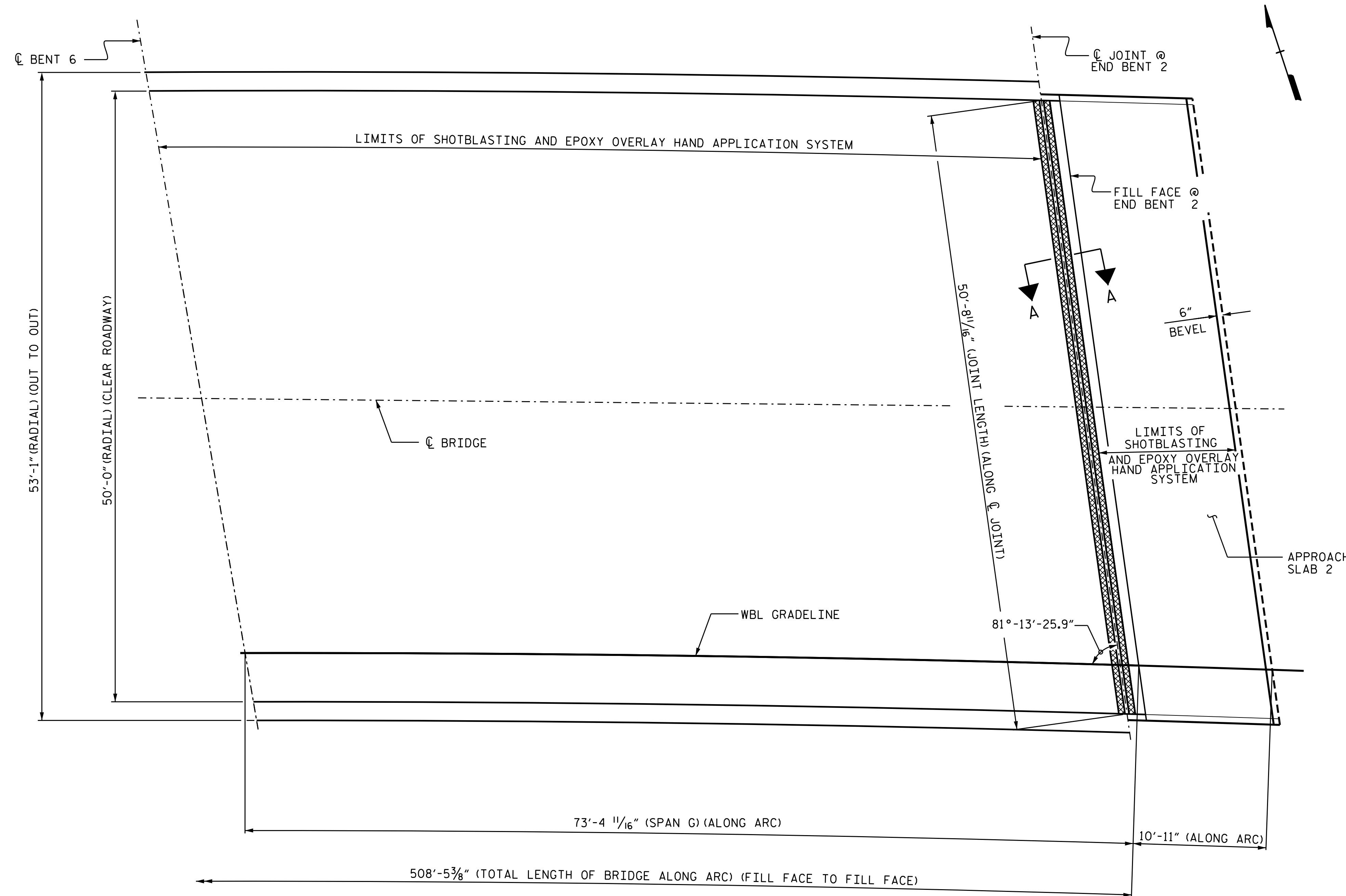
PLAN OF APPROACH SLAB 2 AND SPAN G (SEE SHEET S7-10 FOR SECTIONS A-A AND B-B)
