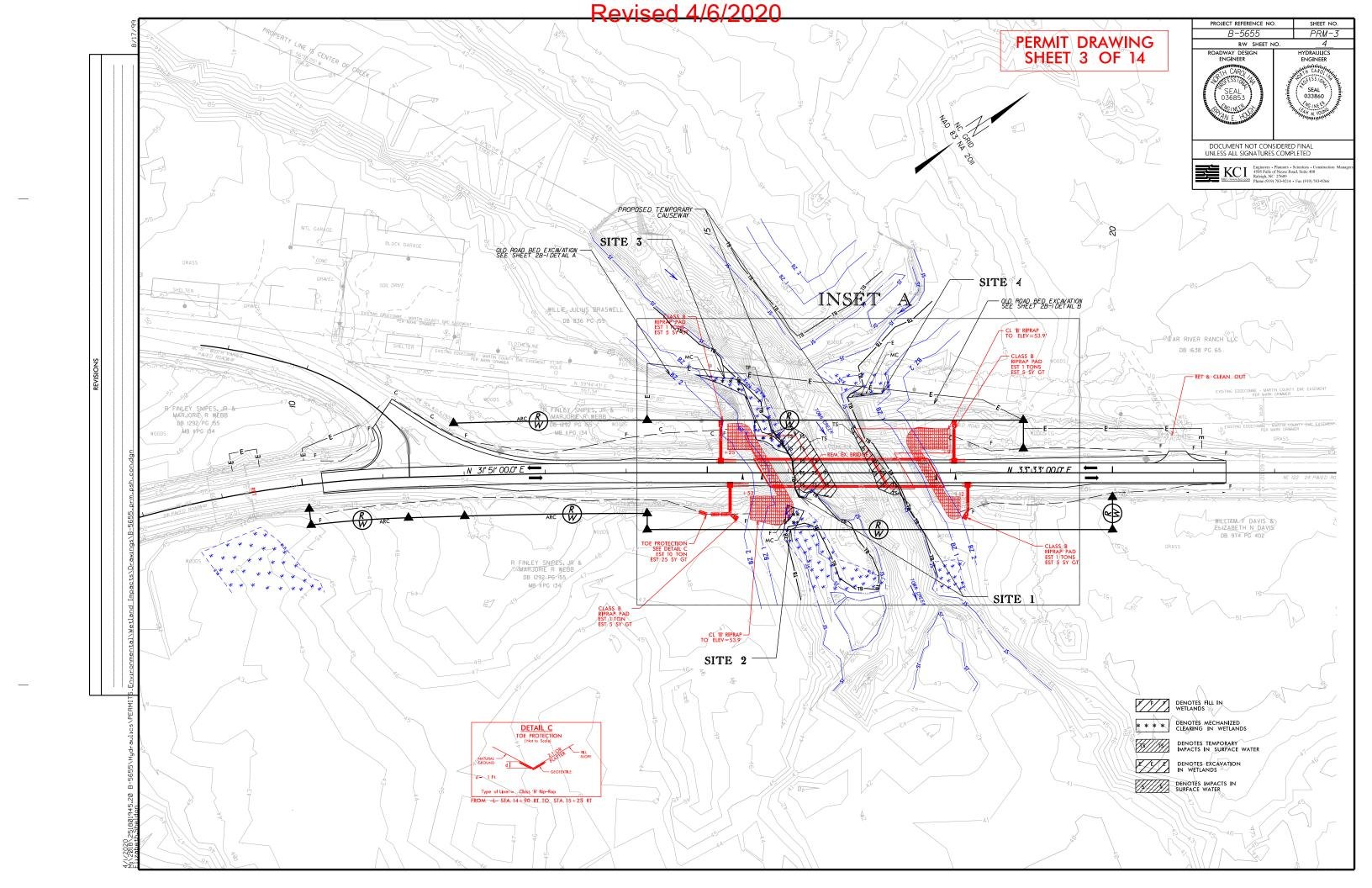
Revised 4/6/2020 SHEET NO. PROJECT REFERENCE NO P<u>RM−</u>4 B-5655 PERMIT DRAWING PROPOSED TEMPORARY CAUSEWAY HYDRAULICS ENGINEER SHEET 4 OF 14 SITE 3 DOCUMENT NOT CONSIDERED FINAL UNLESS ALL SIGNATURES COMPLETED SITE 4 INSET A CL 'II' RIPRAP TO ELEV=53.9' WOODS WOODS **DETAIL C** TOE PROTECTION
