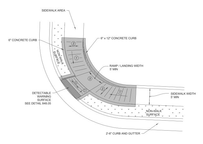
TYPE 3 MODIFIED INSTALLATION IN A RADIUS
