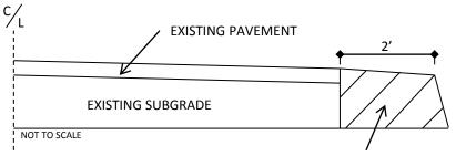
5" ASPHALT CONCRETE BASE COURSE TYPE B25.0B AT AN AVERAGE RATE OF 570 TONS PER SQUARE YARD
