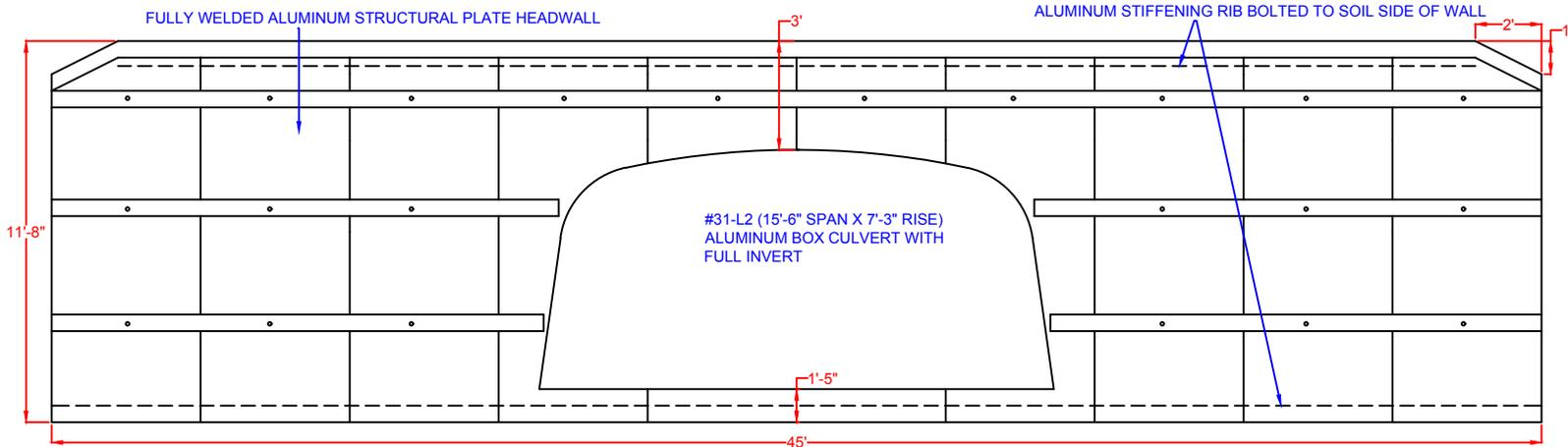
**END VIEW- INLET & OUTLET HEADWALL**
