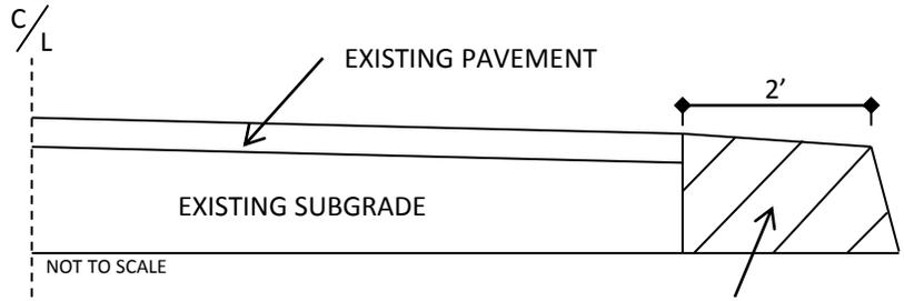
5" ASPHALT CONCRETE BASE COURSE TYPE B25.0C AT AN AVERAGE RATE OF 570 TONS PER SQUARE YARD
