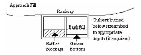
**4.1.3.** Where adjacent floodplain is available, flows exceeding bank-full should be accommodated by installing culverts at the floodplain elevation.
