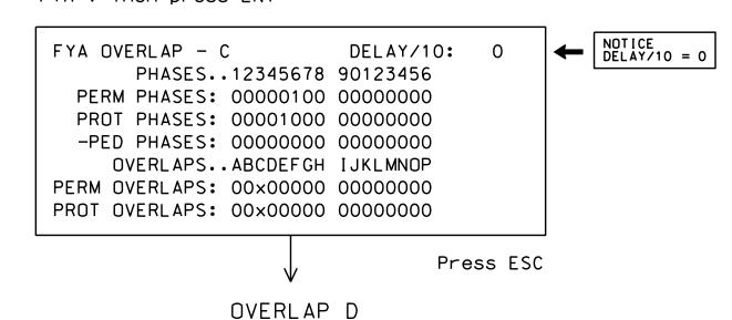
Use Up/Dn/Left/Right keys to position cursor on Overlap 'D'. use the NEXT key to select 'FYA', then press ENT
