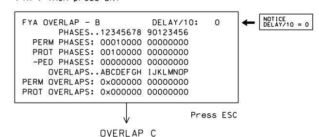
Use Up/Dn/Left/Right keys to position cursor on Overlap 'C'. use the NEXT key to select 'FYA', then press ENT
