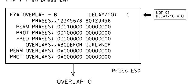
Use Up/Dn/Left/Right keys to position cursor on Overlap 'C'. use the NEXT key to select 'FYA', then press ENT
