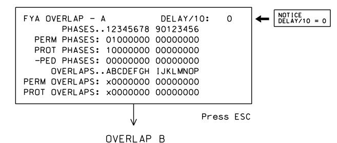
Use Up/Dn/Left/Right keys to position cursor on Overlap 'B'. use the NEXT key to select 'FYA', then press ENT
