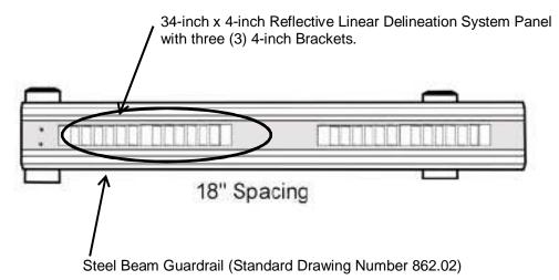
18 inches spacing between each panel into and around curves and a maximum of 36 inches when running parallel with traffic or as directed by the Engineer. Spacing distances may vary depending upon configuration and
