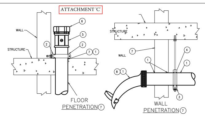
RISER CONDUITS AND SLEEVING END FITTINGS DETAIL
