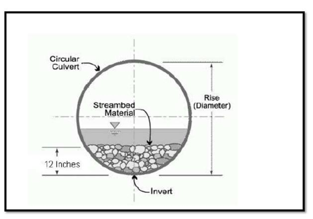
In all other counties: Culverts greater than 48 inches in diameter will be buried at least one foot below the bed of the stream. Culverts 48 inches in diameter or less shall be buried or placed on the stream bed as practicable and appropriate to maintain aquatic passage, and every effort shall be made to maintain the existing channel slope. The bottom of the culvert must be placed at a
