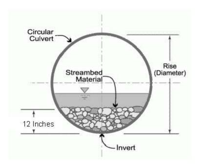
In all other counties: Culverts greater than 48 inches in diameter will be buried at least one foot below the bed of the stream. Culverts 48 inches in diameter or less shall be buried or placed on the stream bed as practicable and appropriate to maintain aquatic passage, and every effort shall be made to maintain the existing channel slope. The bottom of the culvert must be placed at a
