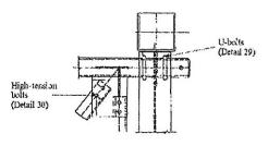
Beam-Cohmun Connection for Truss Structure Example 18
