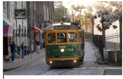
Savannah's trolley system (2009) uses vintage streetcars running on high tech batteries that can also operate with overhead power.
