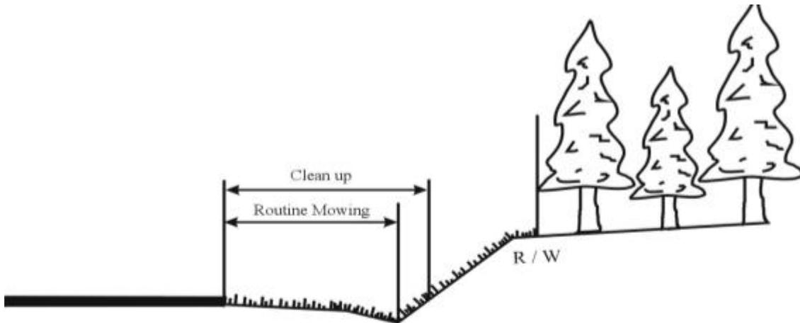
**TYPICAL CUT SECTION WITH SLOPE 2:1 AND STEEPER.**
