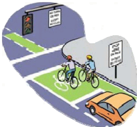
A bicycle box allows bicyclists to position themselves for turns (image: livable streets.org)
