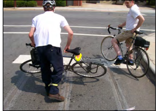
Testing the sensitivity of a loop detector
