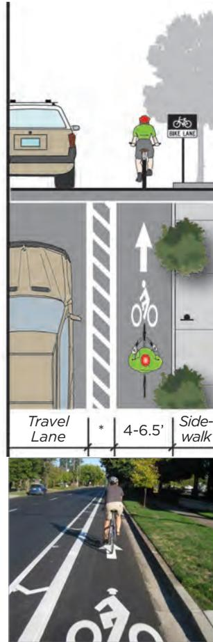
Bike lanes designate an exclusive space for bicyclists, directly adjacent to motor vehicle travel lanes. The preferred minimum width is 6.5 ft to allow bicyclists to ride side-by-side or pass each other without leaving the bike lane. Absolute minimum bike lane width is 4 ft when no curb and gutter is present or 5 ft when adjacent to a curbface, guardrail, other vertical surface or on-street parking stalls (AASHTO [Bike Guide 2012](#)).
