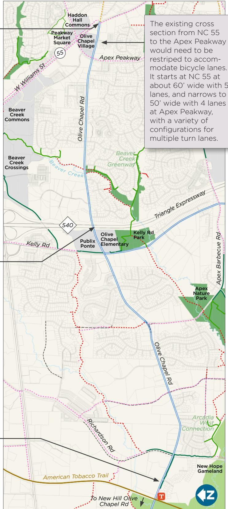
The existing cross section from NC 55 to the Apex Parkway would need to be restriped to accommodate bicycle lanes. It starts at NC 55 at about 60' wide with 5 lanes, and narrows to 50' wide with 4 lanes at Apex Parkway, with a variety of configurations for multiple turn lanes.
