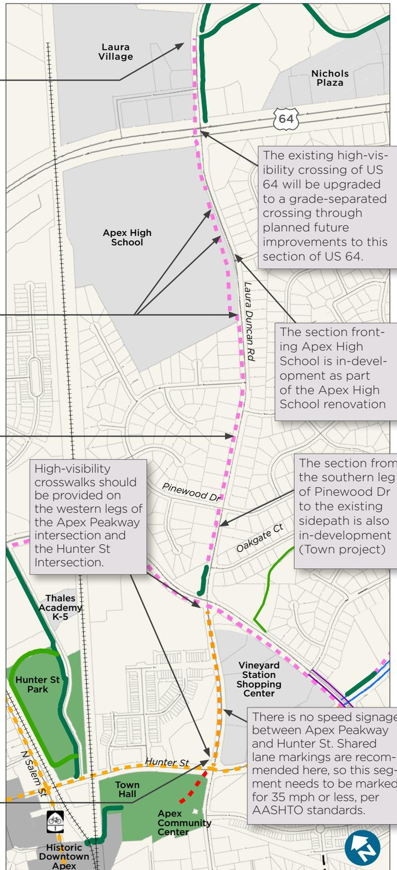
High-visibility crosswalks should be provided on the western legs of the Apex Peakway intersection and the Hunter St Intersection.
