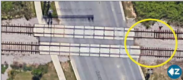
The concrete railroad treatment that closes the flange gap would need to be extended to accommodate the south side side path (in circled area above).
