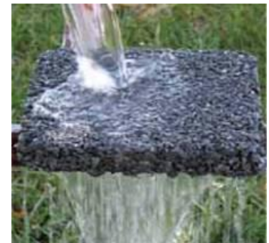
Figure 4-15. Top: Vegetated swale and porous concrete sidewalk help to make a “green street” in the new urbanist development of High Point in West Seattle. Right: Porous asphalt allows the passage of water through small openings, or pores, that are atypical of standard asphalt. Source: Rhode Island Cooperative Extension
