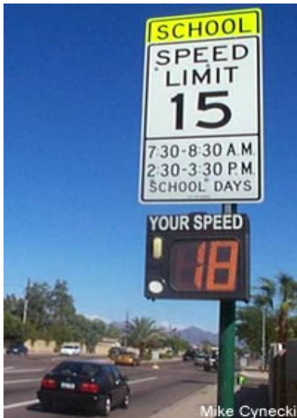
Figure 6-5. Active speed monitors are often used in school zones to discourage speeding. Source: www.saferoutesinfo.org
