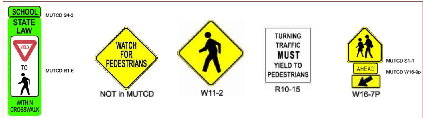
Figure 4-11. Example standard pedestrian warning signs. The first sign (far left) is usually installed within the street to warn motorists to yield to pedestrians in a crosswalk - it does not have to be near a school. The second and third signs are common general pedestrian warning signs, while the fourth and fifth signs notify motorists of specific instances to watch for pedestrians. The fourth sign, “Turning Traffic”, is usually placed at intersections to warn motorists that are turning right or left to yield to pedestrians in crosswalks. For the fifth sign, the top sign can either be combined with the smaller “ahead” sign or the arrow symbol to indicate the presence of a crosswalk to motorists in a school zone.
