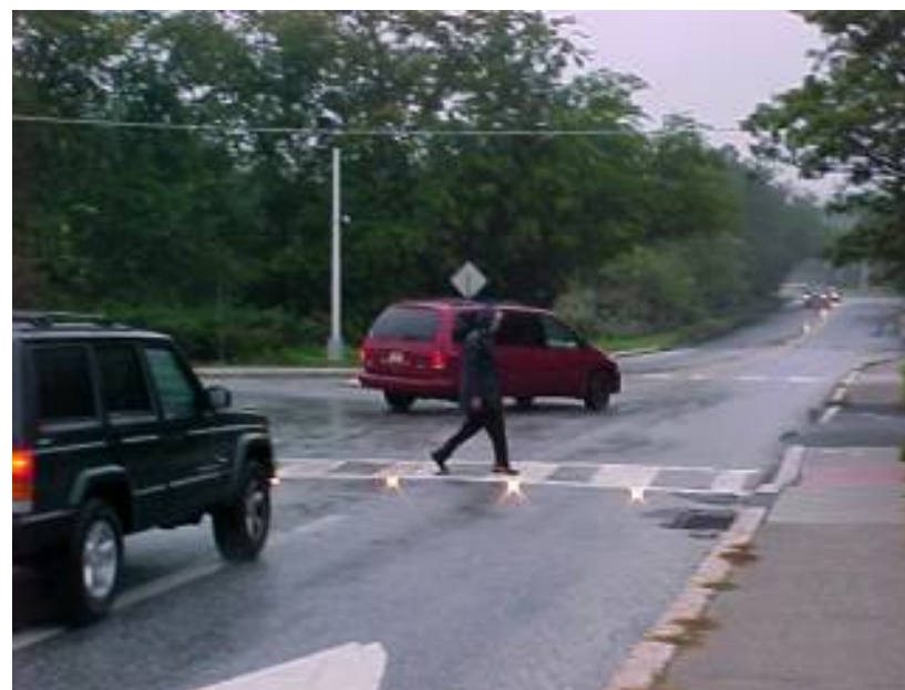
In-pavement flashing warning light system
