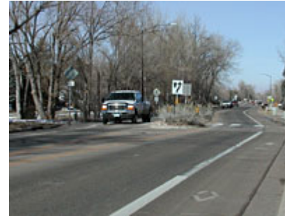
Fig. 5-2: A median refuge on a 3-lane road. Median refuges may be landscaped, but should not obscure drivers' view of pedestrians.
