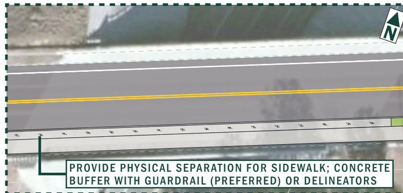
FIGURE 9: BRIDGE WITH PROTECTED SIDEWALK AND FENCING
