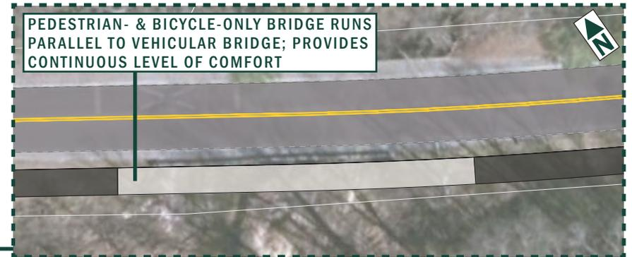
FIGURE 20: ALTERNATE DESIGN DETAIL: CONSTRAINED CREEK CROSSING: TRANSITION TO SIDEWALK ON BRIDGE (1"=100')
