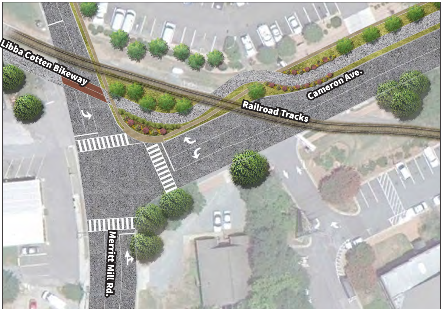
ABOVE: Potential long term reconfiguration of the intersection of Merritt Mill Road and West Cameron to connect Libba Cotten Greenway to West Cameron Ave. Cycle Track.
