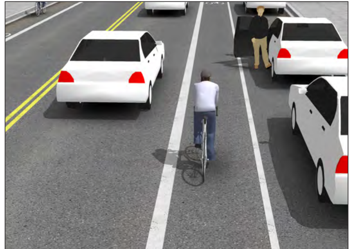
ABOVE: Image from the NACTO Urban Bikeway Design Guide showing an 8 inch solid marking separating the bike lane from the motor vehicle travel lane.
