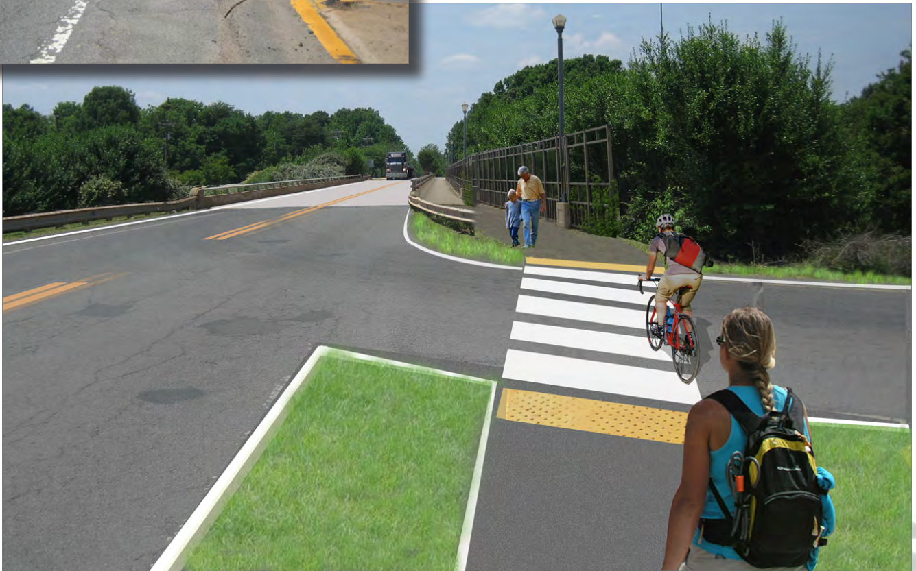
Left: Existing conditions are unsafe for bicyclists and pedestrians at the I-77 bridge and exit ramps. Below: A photo rendering of the same area with a multi-use sidepath across the bridge.
