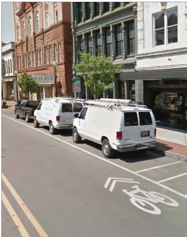
Marked shared roadway (sharrow) example in Downtown Wilmington, NC, on Front Street
