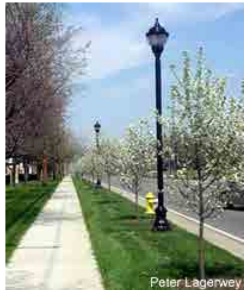
Sidewalks should be a minimum of 5 feet wide and include a landscape buffer with street trees between the road and the sidewalk. Source: Safe Routes to School
