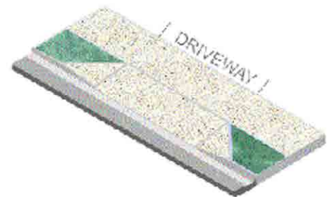
Preferred — The sidewalk is set behind the driveway apron and planting strip.
