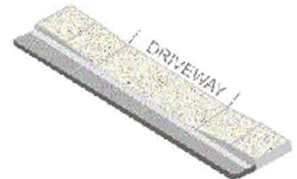
Conditionally Acceptable — The "dip" at the driveway apron allows for safer passage with no cross-slope.
