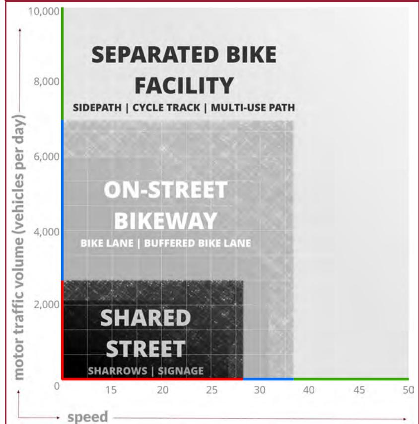
**FIGURE 3.1: GENERAL FRAMEWORK FOR BIKEWAY SELECTION BY VPD AND SPEED**
