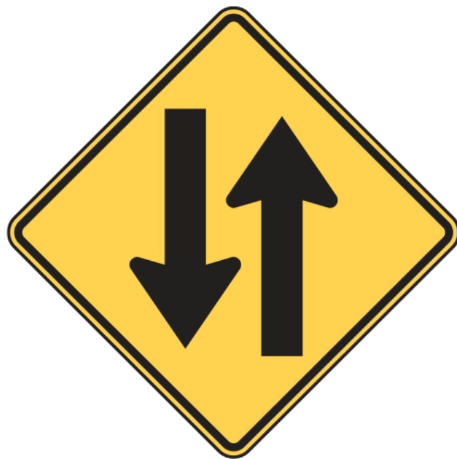
Use a Two-Way Traffic warning sign (MUTCD sign W6-3) to clarify two-way operation of the road if any confusion exists.
