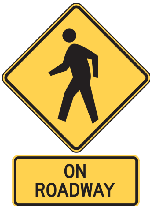
A PEDESTRIAN (MUTCD sign W11-2) warning sign with ON ROADWAY legend plaque.
