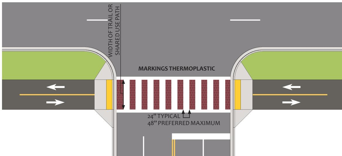
**FIGURE 46: Separated Bike Lane (SBL) Street Crossing**
