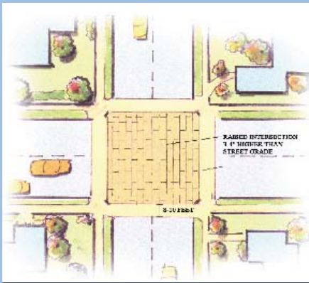
Raised intersection with decorative pavement.
