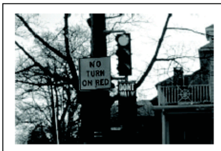
A low cost sign that restricts right-hand turns at a red light. Source: Pedestrian and Bicycle Information Center
