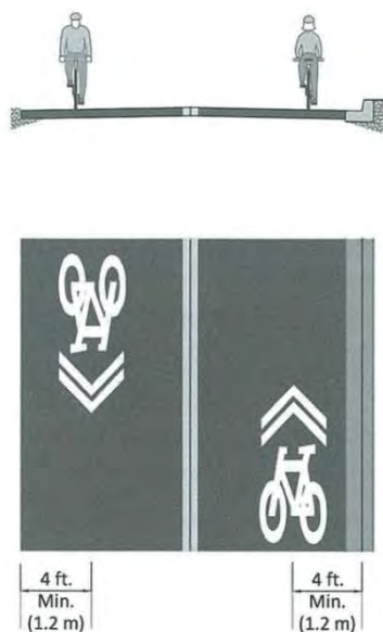
Figure 4-6. Typical Shared-Lane Marking Cross Section on Street with No On-Street Parking
