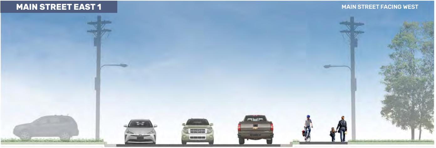
The section from First Street to the crossing of Worrell Mill Swamp has 60' to 65' of right of way and constraints from both structures and topography. In order to economically fit a sidepath in the existing section one option to consider is a narrowing of the travel lanes and shifting the center of the street to the south to allow the sidepath to fit on the north side. Pictures from a similar shift being constructed (Gorman Street in Raleigh) are shown above.
