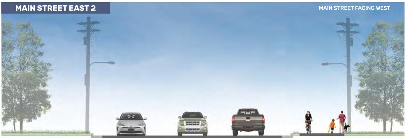
The sections at both the east and west ends of the Main Street project have ample right-of-way to accommodate pedestrian facilities. The existing sidewalk on the north side of the east section could be widened to create a sidepath. The western section also has existing sidewalk on much of the south side to connect to the shopping destinations.
