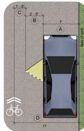
Sharrow Dimensions: A=Distance from Driver Side Door to Face of Curb B=Door Swing Distance C=Distance from Open Door To Centerline of Sharrow Pavement Marking D=Distance from Face of Curb to Centerline of Sharrow Pavement Marking
