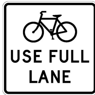
Figure 5.5.3 Use Full Lane Sign for Intersections
