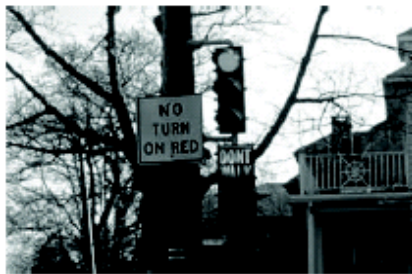
A low cost sign that restrict right-hand turns at a red light. Source: Pedestrian and Bicycle Information Center
