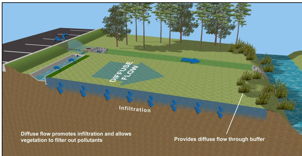
**Figure 3-5.** Typical level spreader configuration and pollutant removal processes
