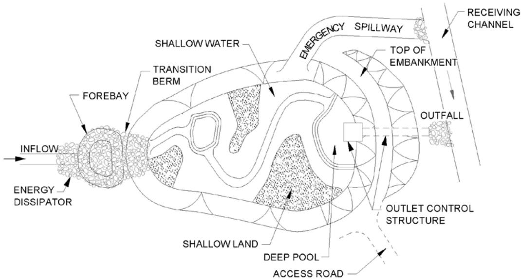
**Figure 13-2.** Profile view: typical stormwater wetland layout and components
