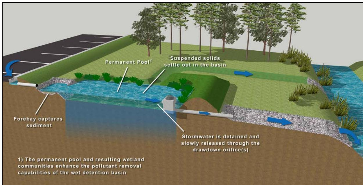
**Figure 12-4.** Typical wet detention basin configuration and pollutant removal processes
