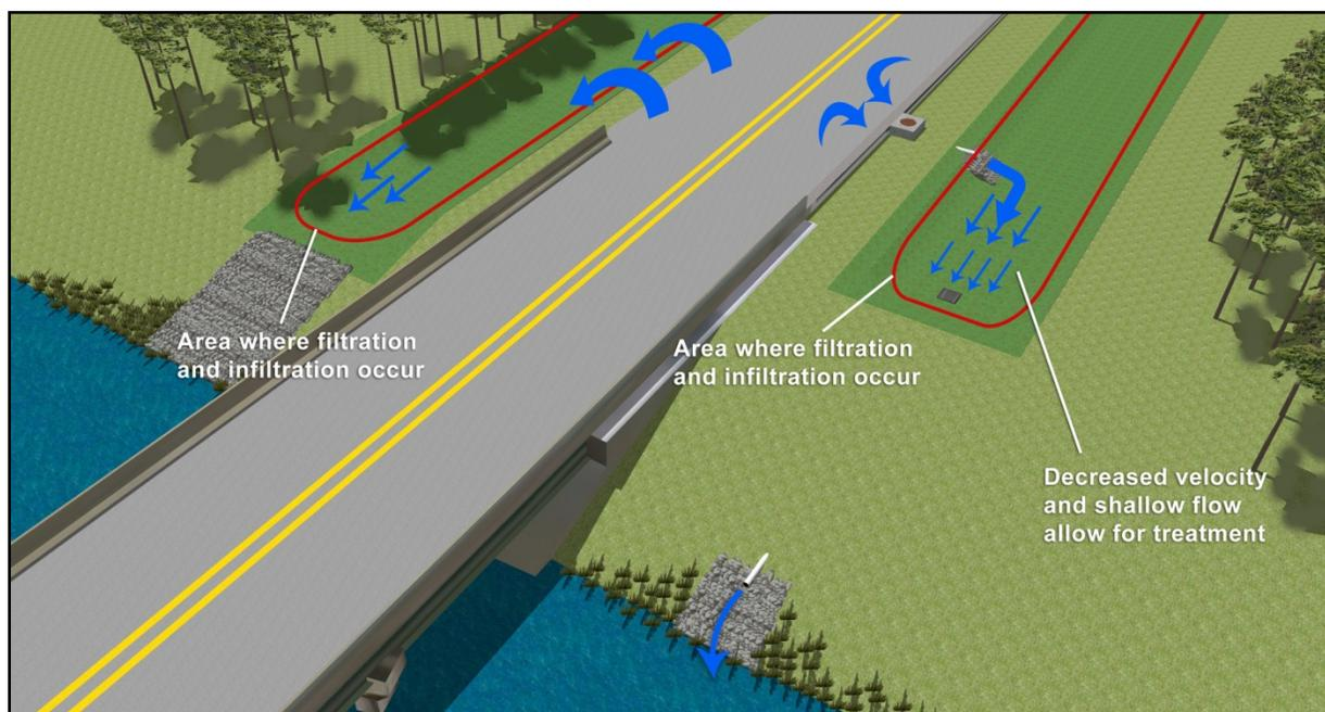
**Figure 6-5.** Typical swale with associated pollutant removal processes
