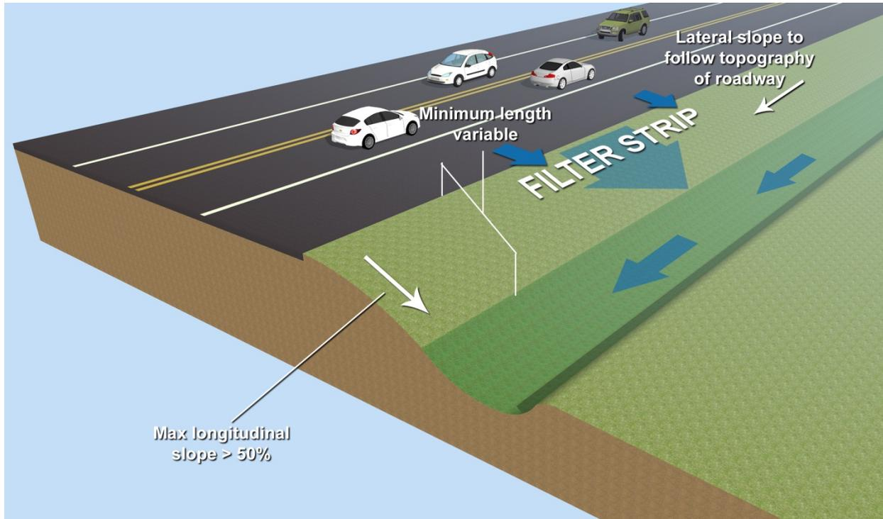
Figure 14-4. Typical roadway filter strip design components
