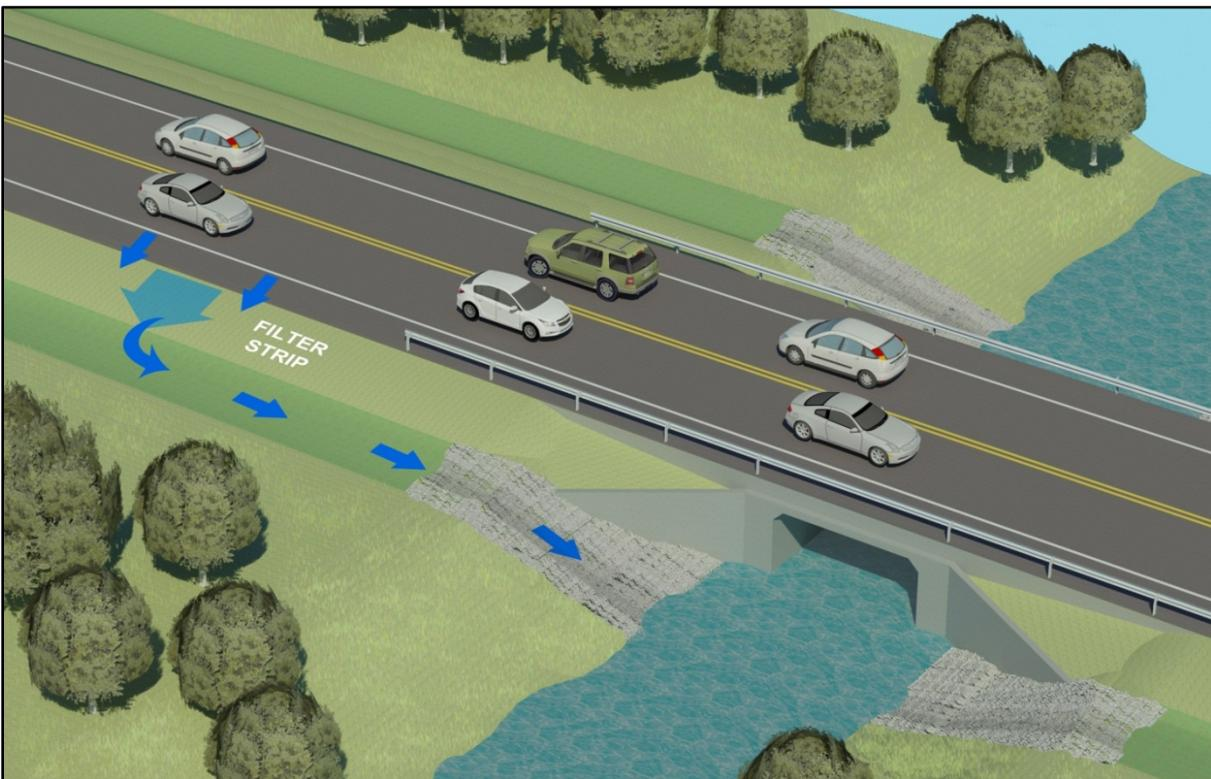
**Figure 14-5.** Example of conveyance designed downstream of filter strip to protect buffer and streambank from erosion
