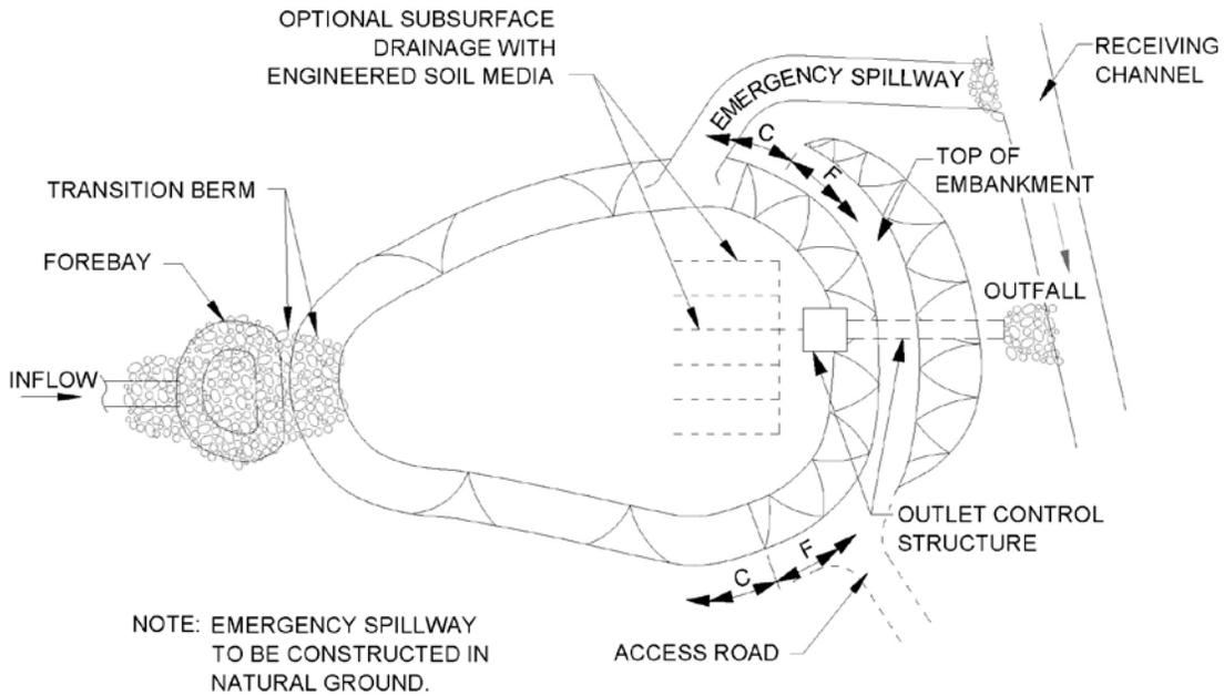
Figure 5-2. Plan view: typical dry detention basin layout and components
