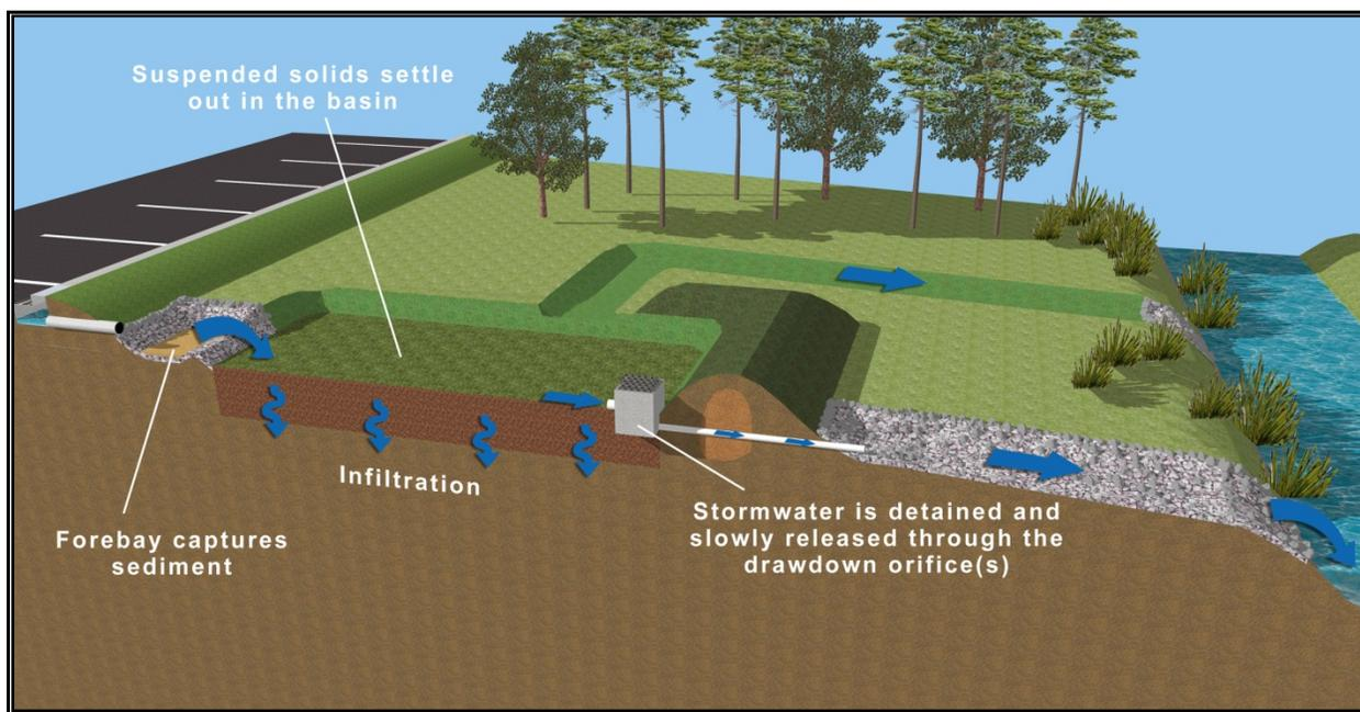
**Figure 5-4.** Typical dry detention basin configuration and pollutant removal processes
