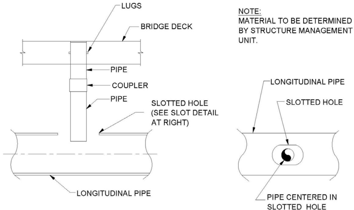
**Figure 9-8.** Elevation view (left) and plan view (right) of deck drain and longitudinal pipe connection
