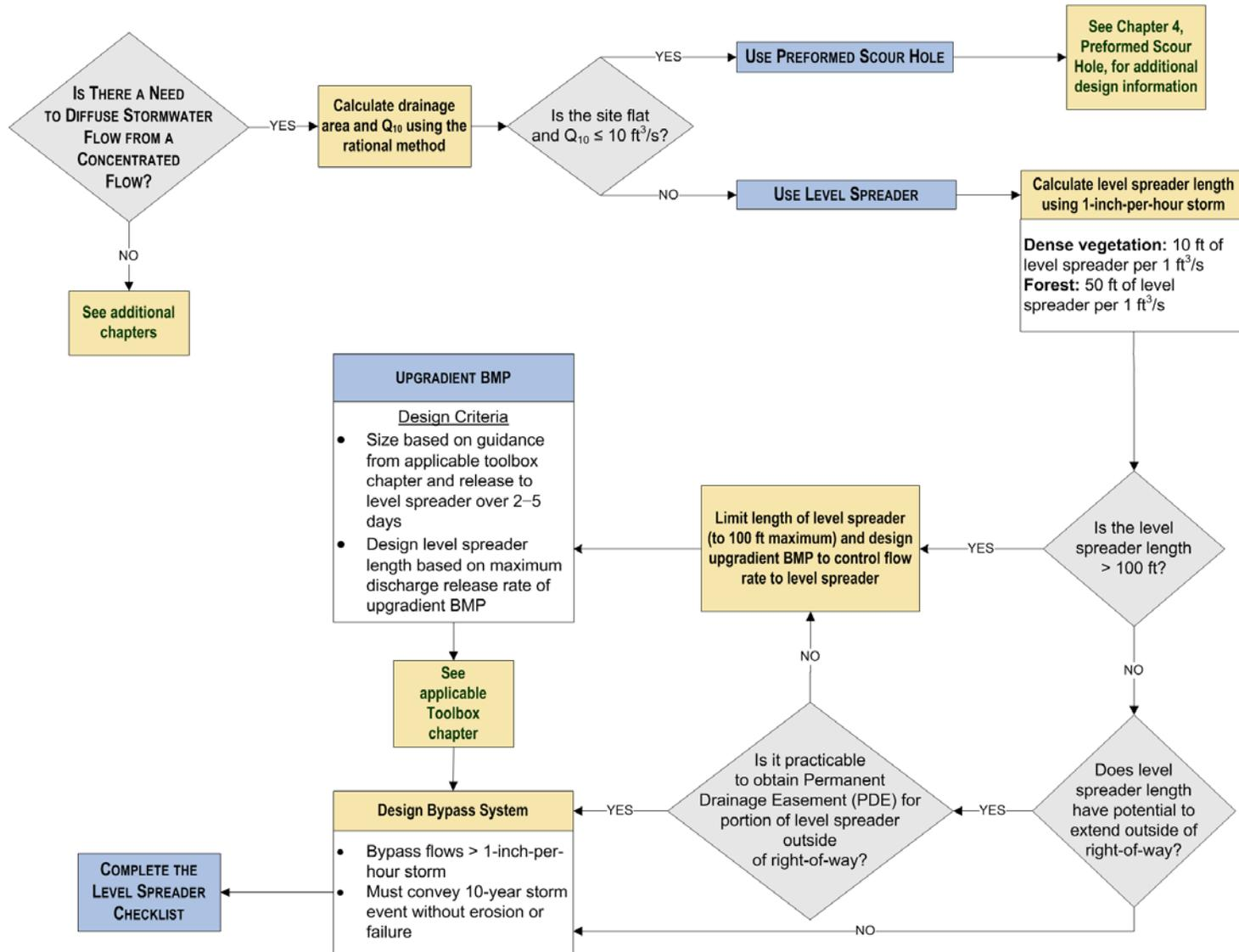
Figure 3-6. Level spreader design flowchart
