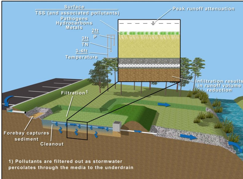
Figure 11-3. Typical filtration basin configuration, pollutant removal processes, and depths required for given constituents
