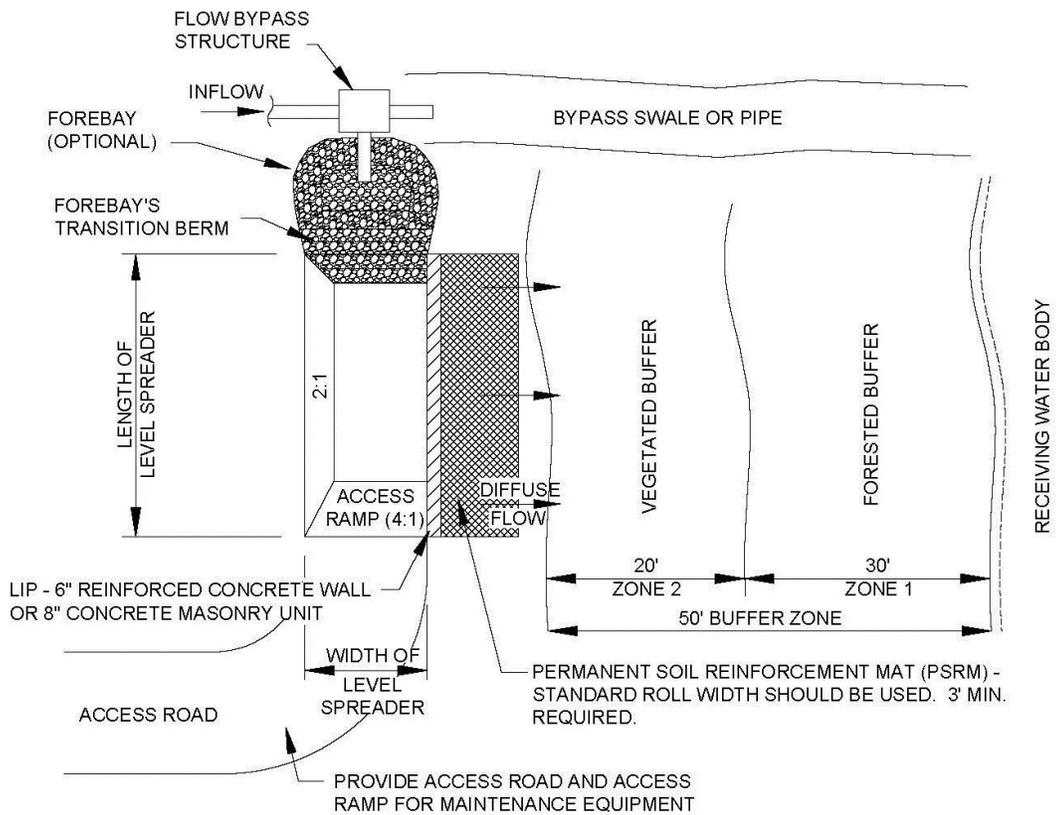
Figure 3-1. Plan view: typical level spreader layout with buffer
