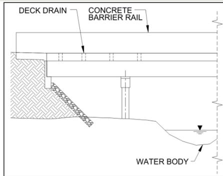
**Eliminate Deck Drains Over Water Body**
