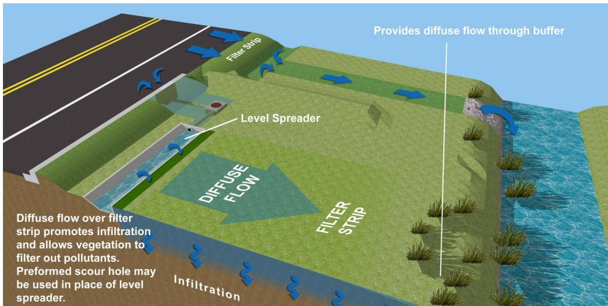
**Figure 14-2.** Typical filter strip configurations and pollutant removal processes
