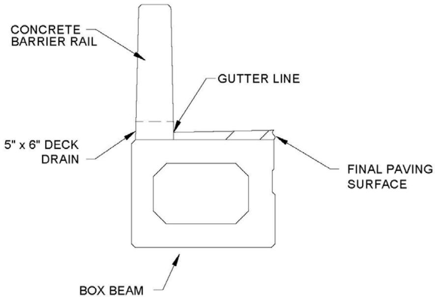
**Figure 9-7.** Deck drain orientation for box beam bridges
