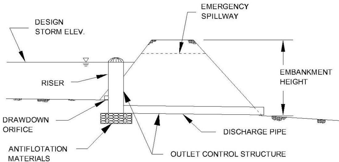
Figure 2-5. Detention basin components
