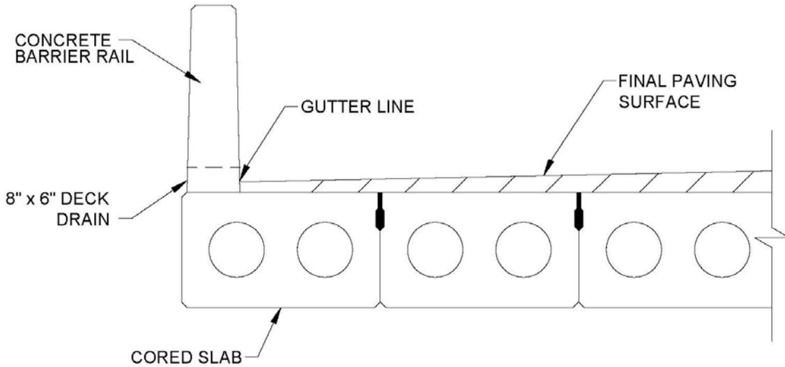
**Figure 9-6.** Deck drain orientation for cored slab bridges
