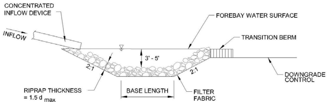
Figure 7-3. Profile view: riprap forebay cross section
