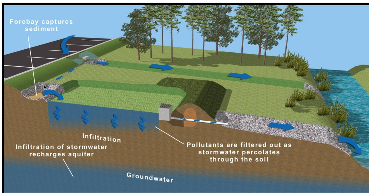
**Figure 10-3.** Typical infiltration basin configuration and pollutant removal processes
