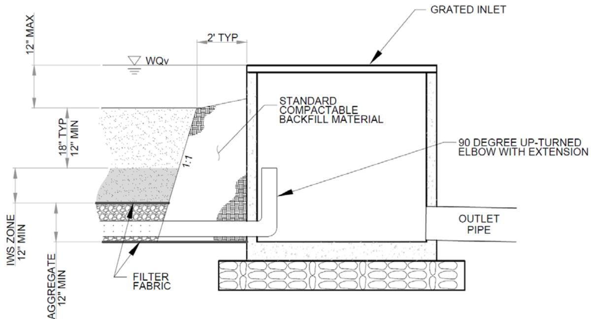
**Figure 11-5.** Profile view: internal water storage zone configuration
