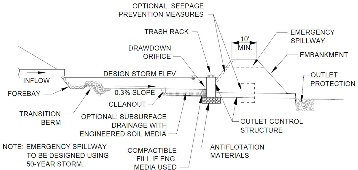
Figure 5-3. Profile view: dry detention basin cross section
