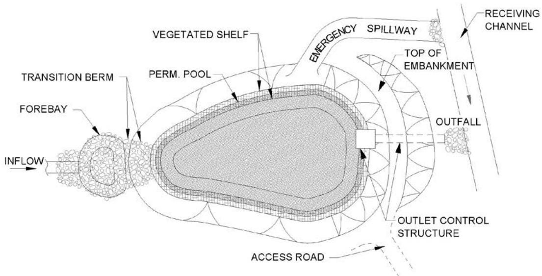
**Figure 12-2.** Plan view: typical wet detention basin layout and components
