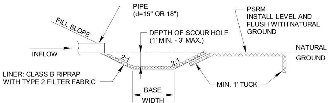
Figure 4-3. Profile view: preformed scour hole cross section
