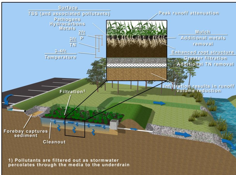
Figure 11-4. Typical bioretention basin configuration, pollutant removal processes, and depths required for given constituents
