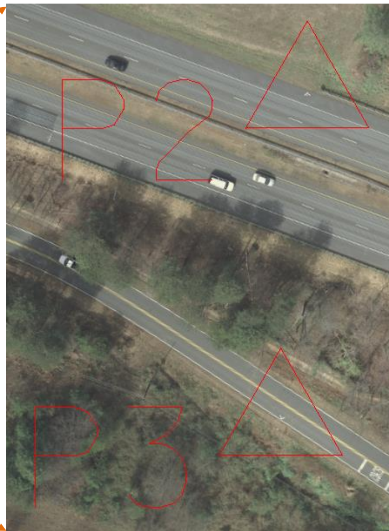
Panel – ground surveyed photo control point
