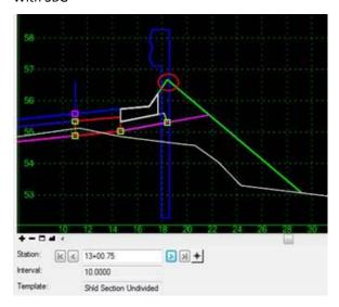
To be consistent with how it is going to be constructed in the field, a couple of key null and normal points have to be added to all templates which have the SBG end conditions.
