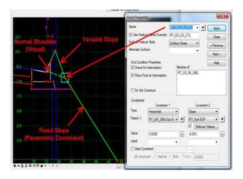
The result is a much smoother seamless transition for a better construction model and more accurate earthwork computation and project footprint/limits of construction.
