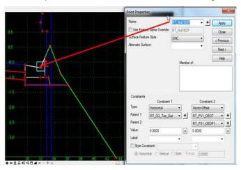
A second point is used as the new shoulder break point occupying the exact location of the edge of usable shoulder point in a normal shoulder situation. This new break point changes the end condition behavior in two folds.
