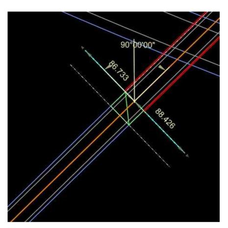
Use the handle at the middle, of the bridge, to adjust the rail offset from the EOT. The bridge civil cells are designed with a uniform rail offset, thus the middle handle is recommended. The handles at the ends will result in an error:
