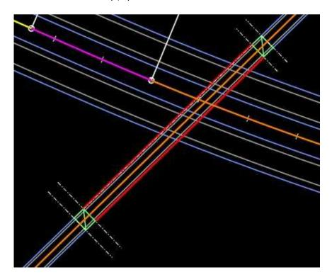
The referenced bridge limits are construction class elements, which will not be printed. Use them as civil geometry elements to change and adjust any of the bridge parameters.
