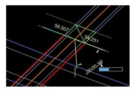
Use the handle at the middle, of the bridge, to move or slide the bridge limits up or down the centerline:
