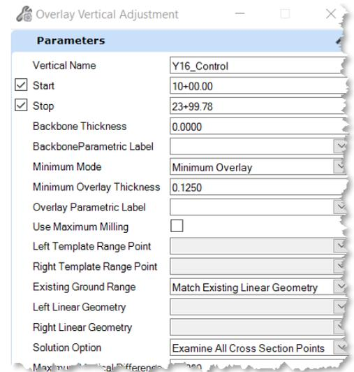
G. After confirming the **Existing Ground Range** parameter and accepting the **Match Existing Linear Geometry** value, you will be prompted to locate the **Left** and **Right Linear Geometry**. At this stage, select the corresponding **Left** and **Right Existing Edge of Pavement** elements, as displayed in the illustration below.
