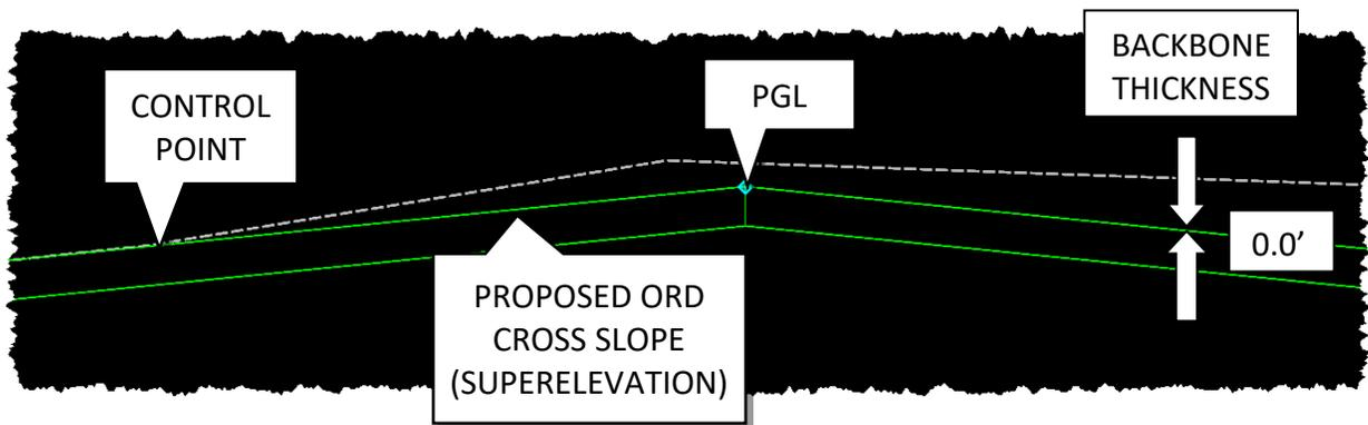
Note: In the image above, the Control Point marks the lowest point along the existing asphalt where it meets the bottom of the backbone. To determine the PGL (Profile Grade Line), we project the Proposed ORD Cross Slope (superelevation) from the Control Point toward the centerline of the roadway. The superelevation (variable) is applied based on project-specific settings, not template defaults.
