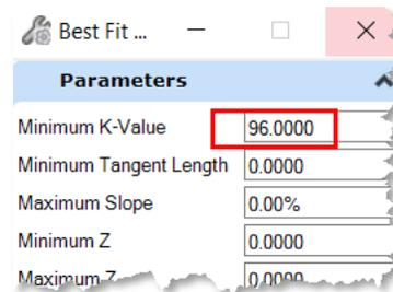
Note: This tool was not specifically designed for this application; because of this, only two parameters are relevant in this context, while the others are disregarded. Additionally, since there is only a single K-value parameter instead of separate values for sag and crest curves, you should select the worst-case scenario of the two based on your design criteria.
