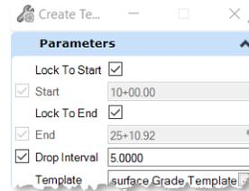
Note: NCDOT recommends using a 5' drop interval when utilizing a corridor to develop a grade because it will provide very accurate data.
