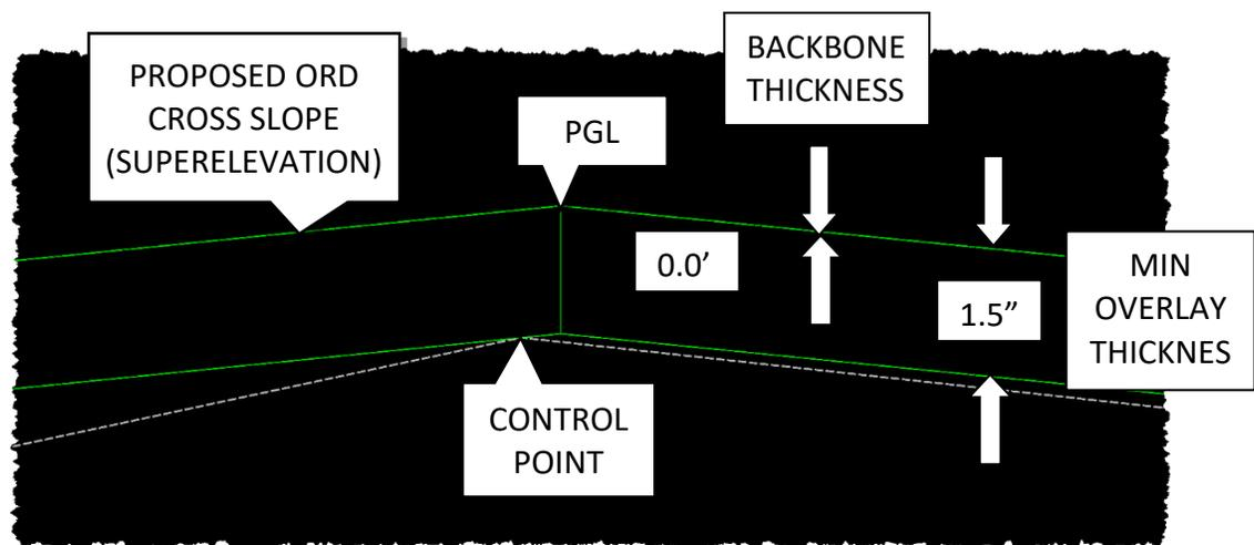
Note: In the image above, the control point marks where the bottom of the 1.5-inch Minimum Overlay Thickness meets the existing asphalt, with the backbone thickness at 0.0' in this example. To determine the PGL (Profile Grade Line), we add the 1.5-inch overlay thickness to the control point's elevation and project the Proposed ORD Cross Slope (superelevation) toward the centerline of the roadway. The superelevation (variable) is applied based on project-specific settings, not template defaults.
