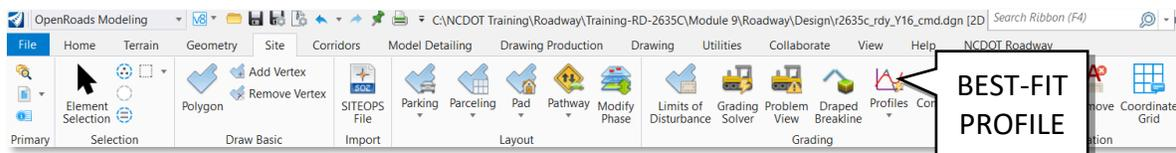
It is important to clarify that the **Best-Fit Profile** tool located under (**Site > Grading > Profiles > Best-Fit Profile**) is distinct from the similarly named **Define Profile by Best Fit** tool found under (**Geometry > Vertical**). The **Define Profile by Best Fit (Geometry > Vertical)** tool offers limited utility and is not recommended for this purpose.
