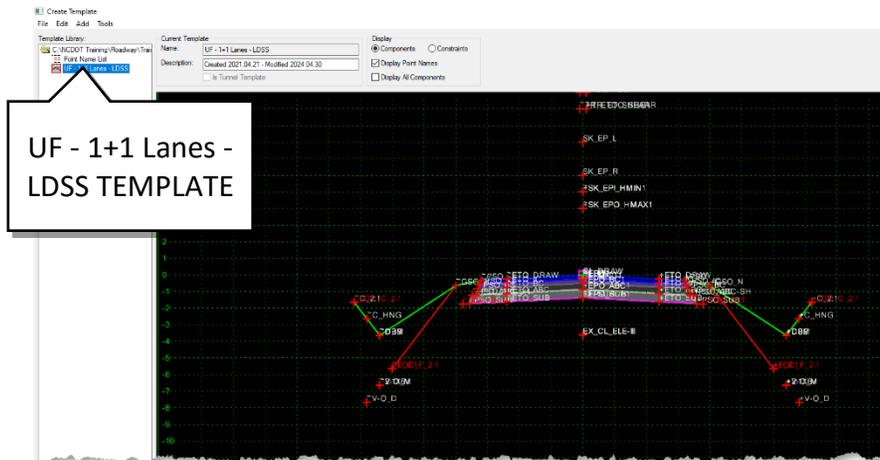
Note: No specific template is required for this exercise. However, it is recommended to choose a template that closely aligns with the intended design, particularly in relation to the pavement and PGL (Proposed Grade Line). Understanding the differences between a divided and undivided facility is crucial in this context. Once you have established a working grade, there is no need to maintain the same template throughout the duration of the project.
