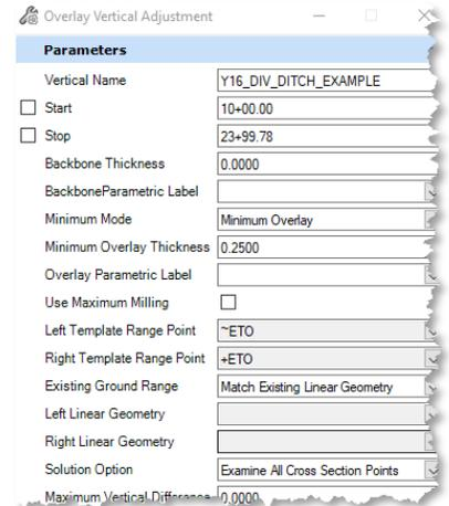
G. After confirming the **Existing Ground Range** parameter and accepting the **Match Existing Linear Geometry** value, you will be prompted to locate the **Left** and **Right Linear Geometry**. At this stage, select the corresponding **Left** and **Right Existing Edge of Pavement** elements, as displayed in the illustration below.
