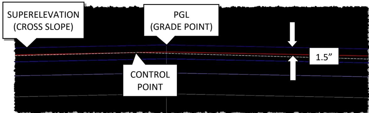
Note: It is important to recognize that the Overlay Vertical Adjustment tool incorporates various parameters in addition to the ones used in this particular exercise. Ultimately, the goal is to develop a proposed PGL elevation that aligns with the pavement design criteria. Multiple combinations of these parameters can yield the same proposed PGL elevation.
