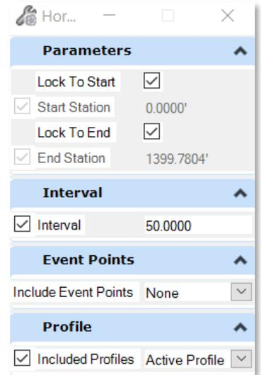
Note: The Interval is used to determine a stationing interval for reporting purposes. This should be set based on the need.
