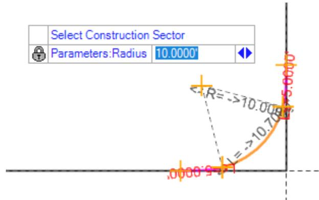
H. Left click to accept the Trim option of Both. This will complete the tool and place the Spiral Curve Spiral combination. This also trims the reference elements to the spiral transitions.
