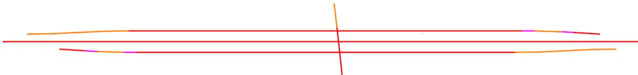
BBB. The last step is to set the tangent lengths required. This would normally be done in conjunction with the ramp and loop designs. For this design we know that the tangent length to the Left of Y8 Should be 1791.14' and to the right should be 2235.16. Use the element selection tool to highlight the central tangent and active the text manipulators.
