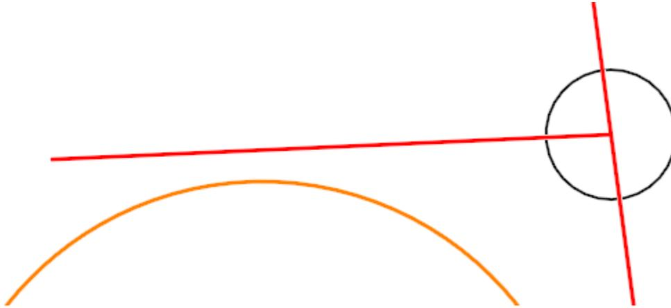
P. The next step is to construct a curve with a radius of 600.00' that is 20.00' offset from the Loop centerline. Start the **Arc Between Elements** tool.
