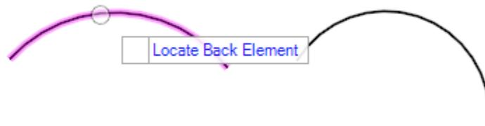
H. Left click to accept the Start Offset = 0.00'. Note that the entire circle is shown as a dashed element because the solution can be placed anywhere on the extension of the original arc, not just the portion of the arc in the dgn file.
