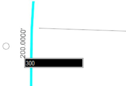
R. The first curve should now have a radius of 4000.00' with a begin and end spiral transition with a length of 300.00'
