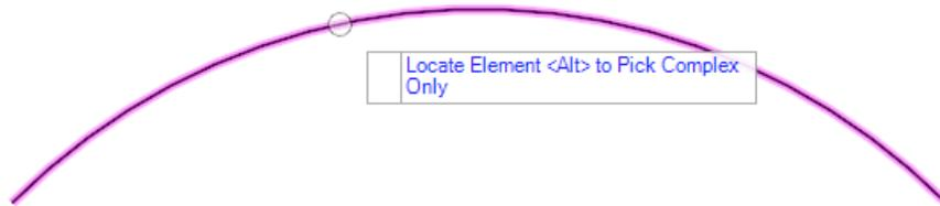
E. The user will be prompted to select a start point. The dynamic display shows two dashed elements. One dashed element represents the extension of the From element arc. The solution can be anywhere on the extension. The other dashed line represents the projection of the cursor location to the From element arc. Note that the offset is locked to 0.00' and the proposed line will start on the element not where the cursor is located.
