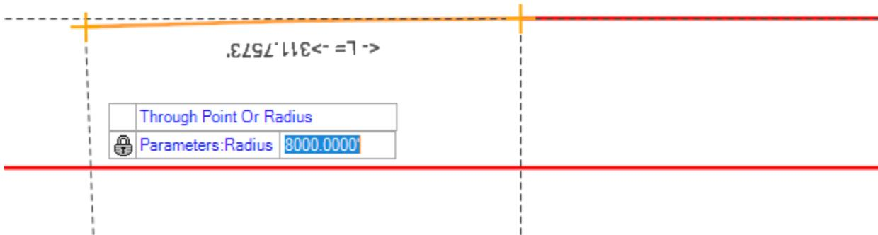
OO. Left click to dynamically accept an Arc Length. This length can be any value. During the placement of the reversing curve the trim option can be set to back and the curves will adjust to tie at the tangent point.
