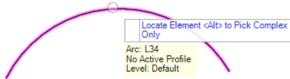
H. Left click to set the start point. This is the point on the From Element where the transition curve will tie tangentially. This can be done by snapping to a point on the From Element or by snapping in space. The dashed black line shows the project to the From Element. Note that the start point can be selected anywhere on the projection of the From Element.
