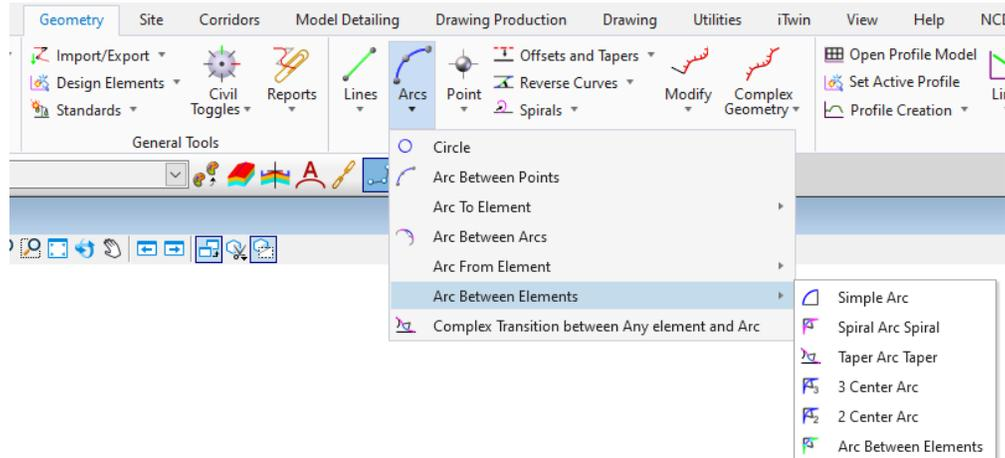
This group contains tools that will allow the user to construct an arc between two previously placed elements. This tool has the ability to optionally apply a back and/or forward transition and/or taper between the elements and the constructed arc. This tool group will be commonly used by the roadway designer.
