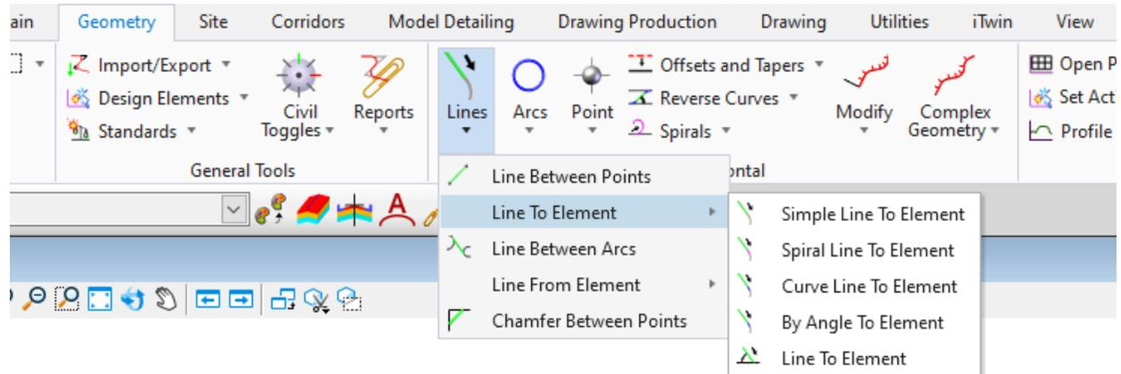
This group contains tools that will allow the user to draw a line segment that will be based on another element. These tools will be used when construction Horizontal Alignments, especially for construction Y Lines, Intersections, Ramps and Loops. Additionally this group of tool will be used when constructing other civil geometry features that will be covered in other Modules.
