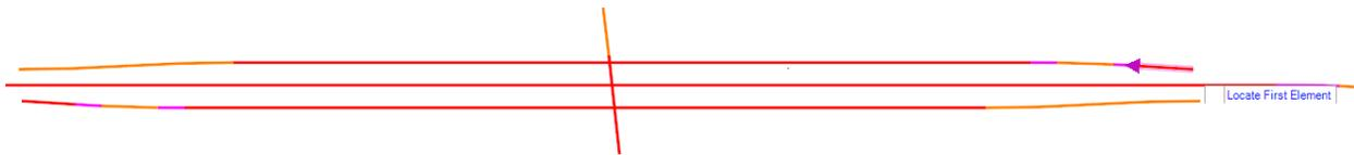
HHH. All the connecting elements will highlight. Left click to accept the complex element. This will create the Complex Element (Geopak Alignment) and complete the tool
