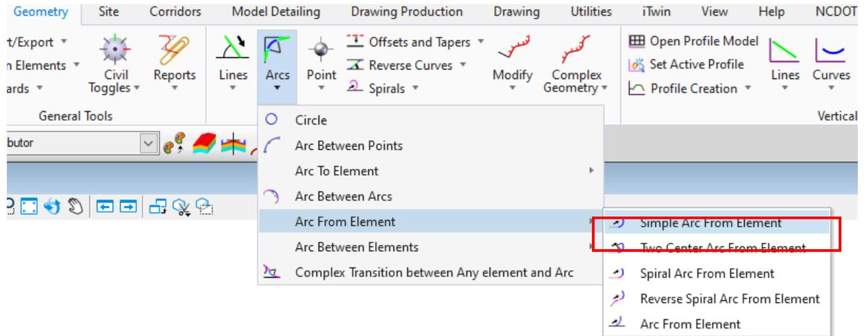
LL. Left click to locate the central tangent of the Collector Distributor alignment
