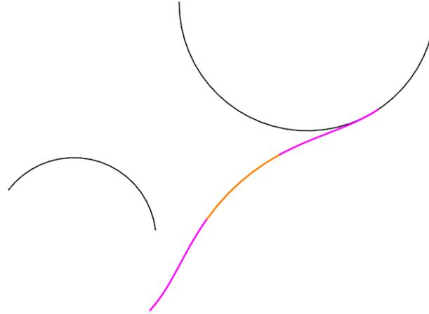
Z. Use the Element Selection tool to highlight the element and note that the spiral ties 2.00' offset from the project of the Back Arc. There are reversing spiral transitions at each end and an arc with a radius of 20.00' in the middle.
