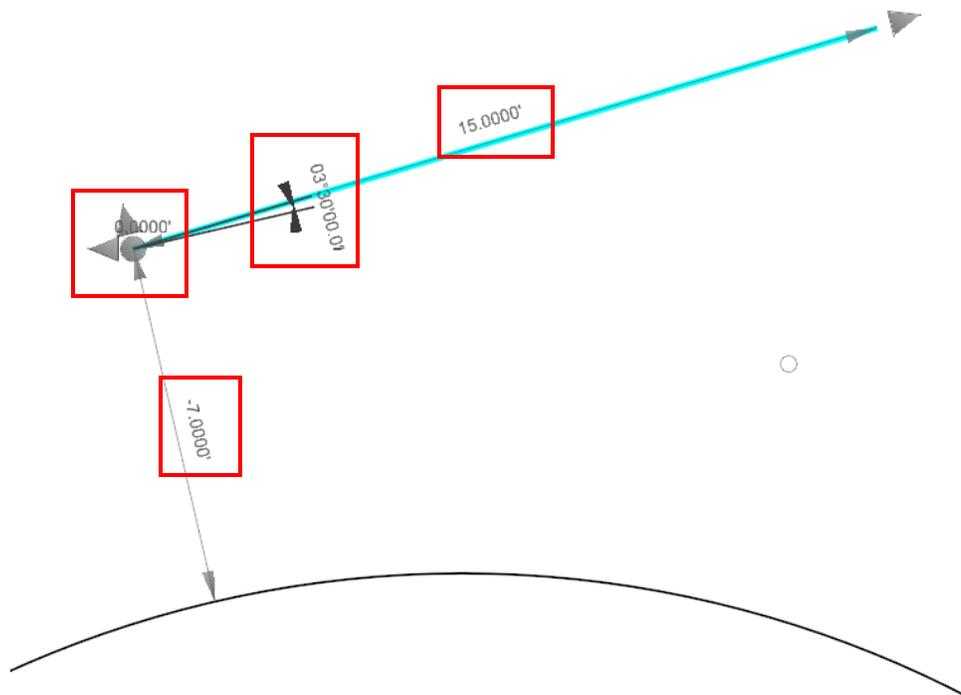
N. This line now starts at a point  $7.0'$  to the left of the From Element at a skew of  $3^{\circ}30'00''$  and has a total length of  $15.00'$
