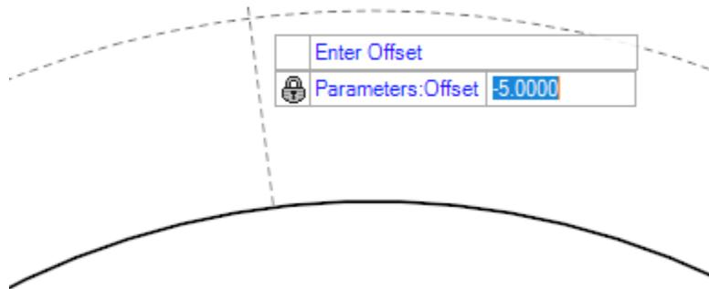
G. Left click to select the Start Point, this is not the start point of the line, this is point where the tool starts the construction of the line. The line will pass through this point. This point will be located at the specified offset from the From Element.
