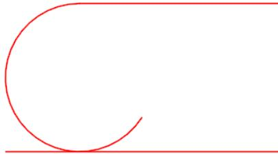
X. Switch to the **Drawing** ribbon and use the **Trim to Intersection** tool from the **Modify** group to trim the end of the curve to the outside line.
