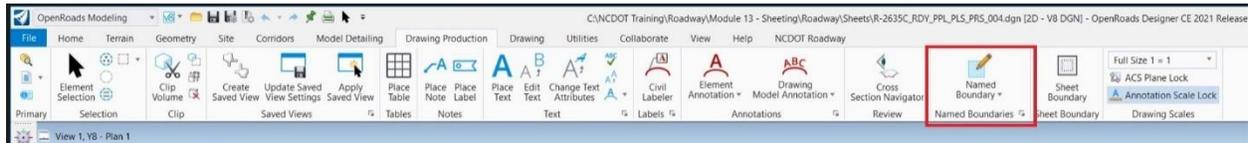
One of the tool groups of the *Drawing Production* Ribbon Tab is the *Named Boundaries* Tool Group. Choosing the tools in this group will place or adjust the named boundaries (clip area shapes) to create plan, profile, and cross section sheets. Note currently adjusting the named boundaries is only applicable to profiles.
