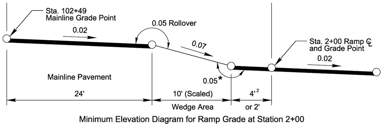
Minimum Elevation Diagram for Ramp Grade at Station 2+00
