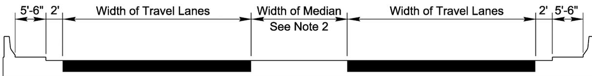
Dual Structure - Curb and Gutter Approach<sup>3,4</sup>
