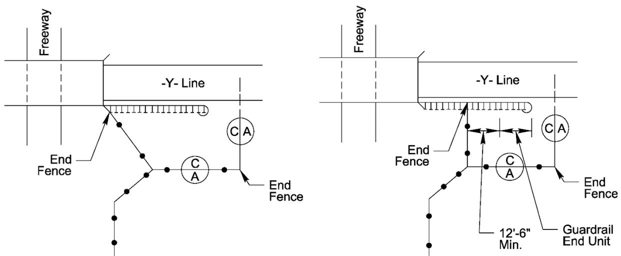
Figure 14-8 Guide for Fence Locations at Freeway over -Y- Line
