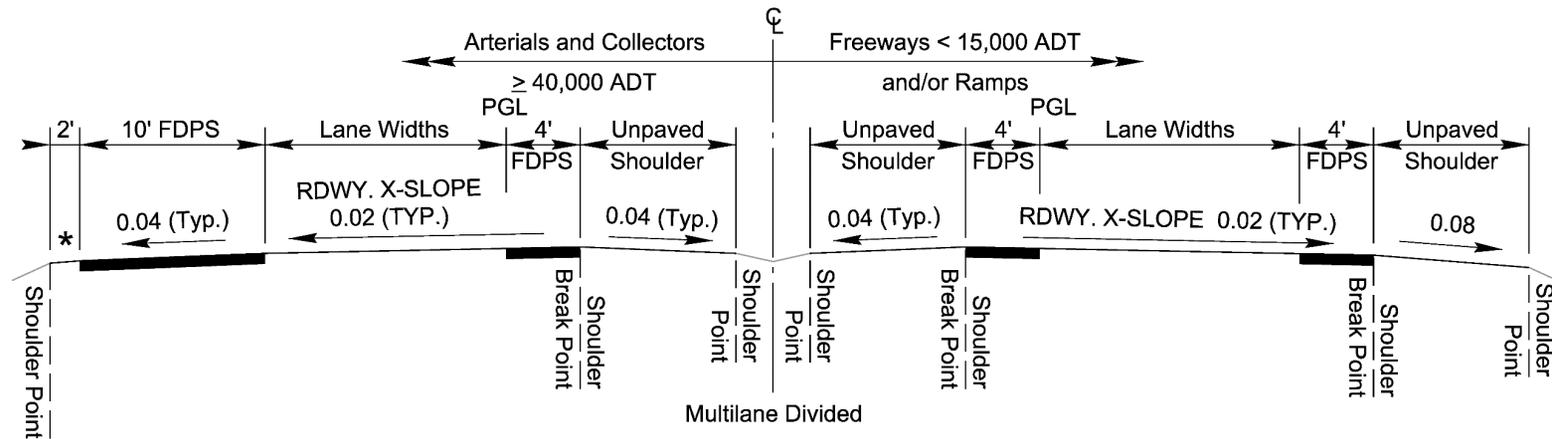
Figure 4-3 Typical Shoulder Cross Slopes (cont.)
