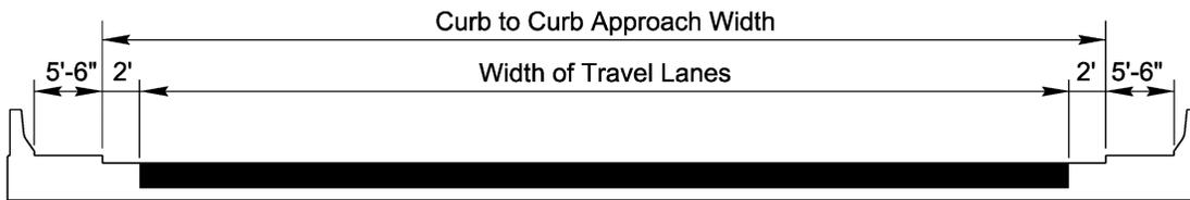
Curb and Gutter Approach With Auxiliary Lanes<sup>4,5</sup>
