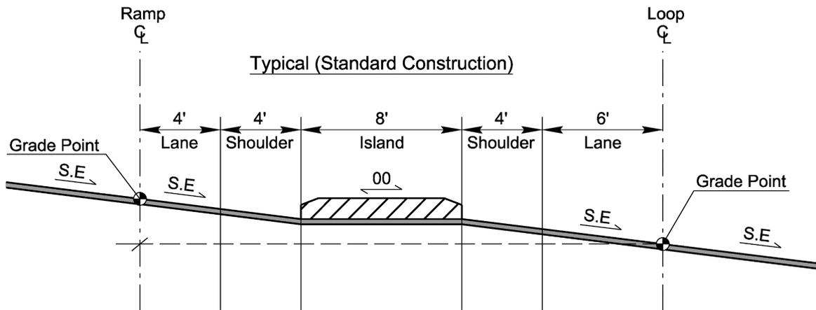
Note: In typical scenario the island is constructed at 0.0% cross-slope.
