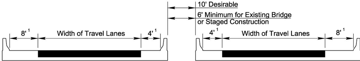
Single Structure - Curb and Gutter Approach<sup>3,4</sup>
