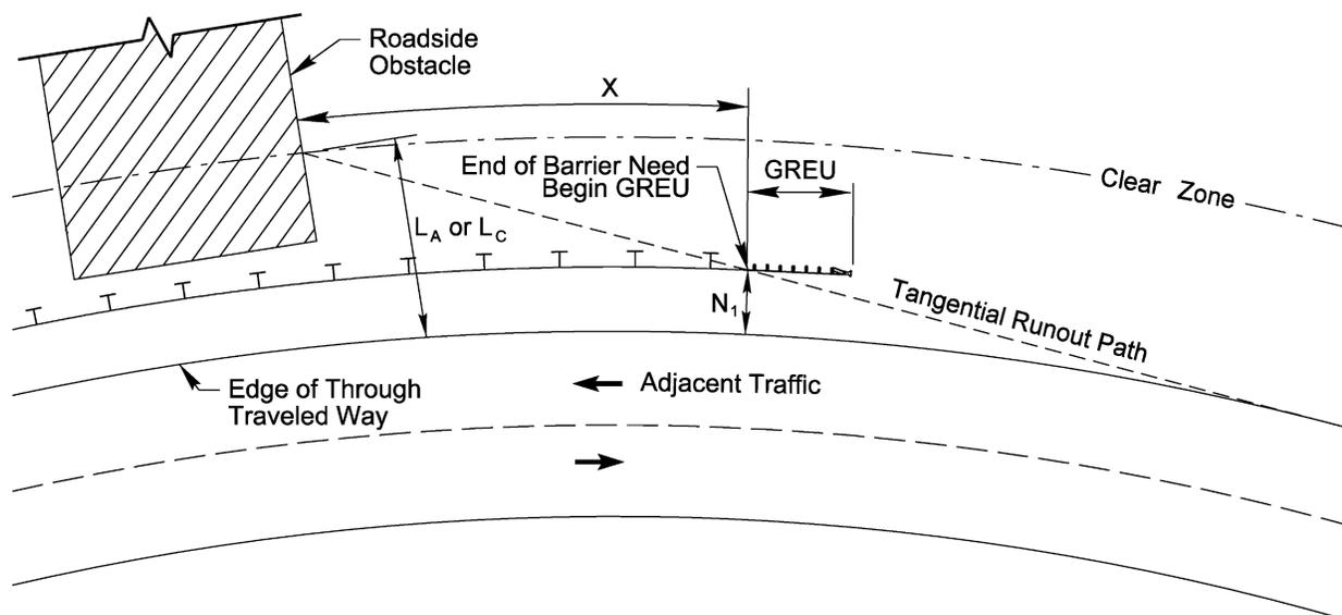
Note: Use  $L_A$  if the roadside obstacle is contained within the limits of the clear zone. If the roadside obstacle extends beyond the limits of the clear zone,  $L_C$  shall be used.
