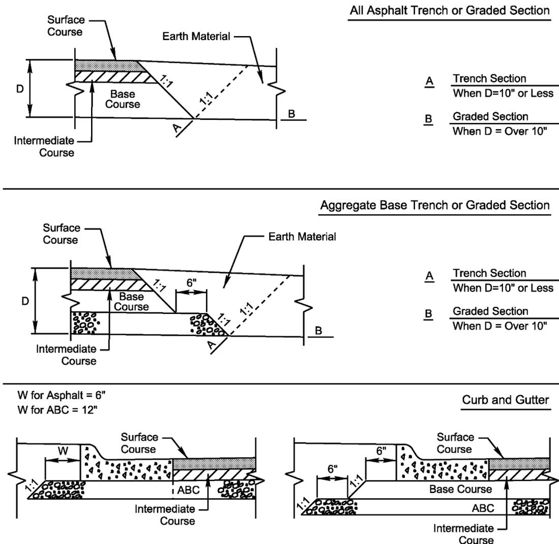
All Asphalt Trench or Graded Section
