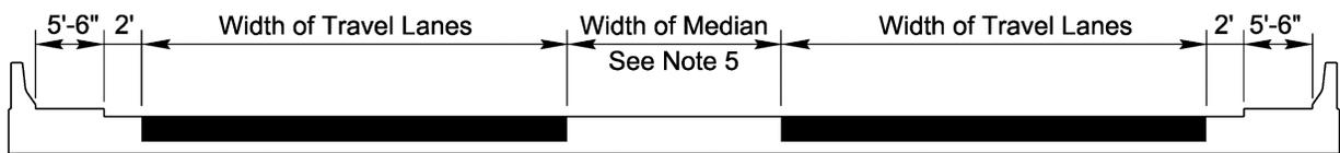
**Dual Structure - Curb and Gutter Approach<sup>6,7</sup>**
