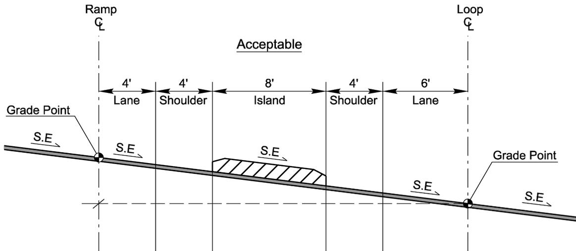
Note: In acceptable scenario the island can be superelevated to match the adjacent roadway cross-slopes.
