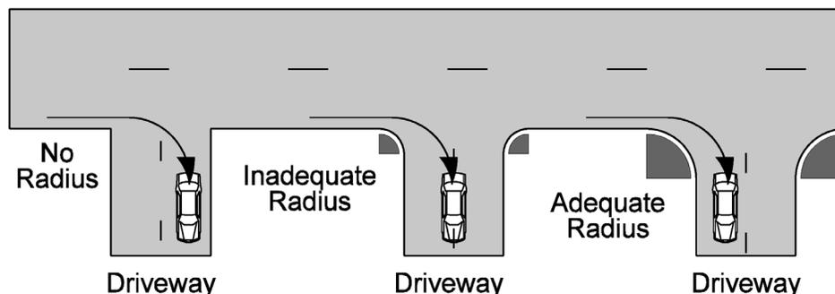
Note: An adequate radius allows turning vehicles to access the site readily and minimizes the impact to the through movement.
