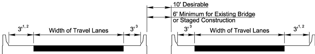
**Single Structure - Curb and Gutter Approach<sup>6,7</sup>**
