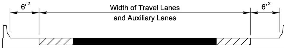
Curb and Gutter Approach Without Auxiliary Lanes<sup>3,4</sup>
