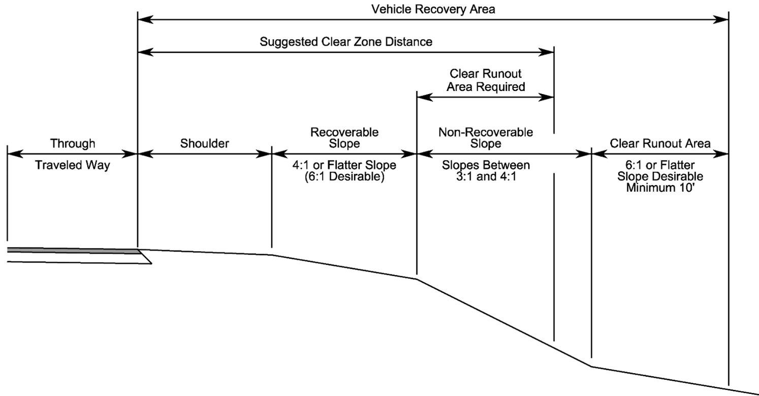
Note: Clear runout area is additional clear zone space that is needed because a portion of the suggested clear zone distance falls on a non-recoverable slope. The width of the clear runout area is equal to that portion of the clear zone distance located on the non-recoverable slope.
