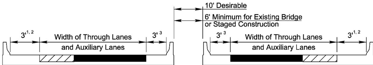
Single Structure - Curb and Gutter Approach<sup>6,7</sup>
