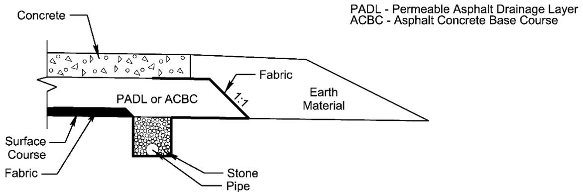
Note: The detail above serves as an example of what a roadway designer may receive from the Pavement Design Unit upon being notified that shoulder drains should be included in the plans.
