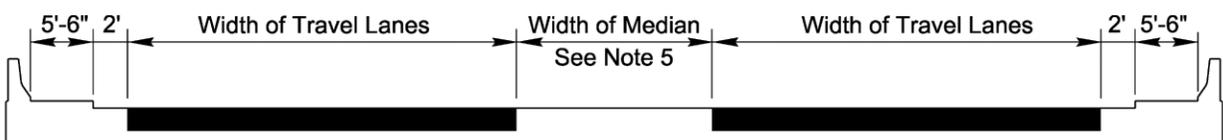
**Dual Structure - Curb and Gutter Approach<sup>6,7</sup>**
