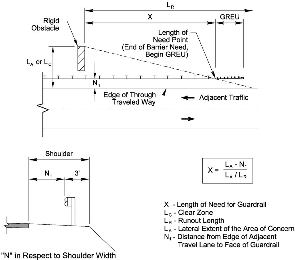
Note: For normal shoulder widths refer to RDM Part I Chapter 4 Section 4.4 Tables 4-1 and 4-2. Note that the width of the shoulder from the edge of travel lane to the face of guardrail increases in certain scenarios as defined in Chapter 4.
