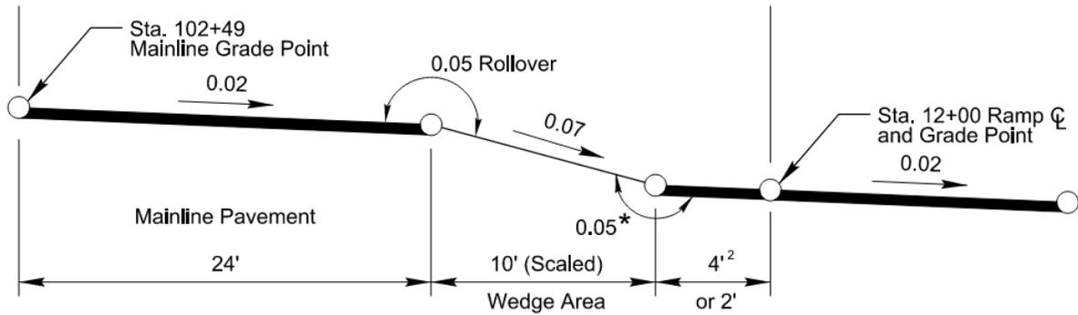
Minimum Elevation Diagram for Ramp Grade at Station 12+00
