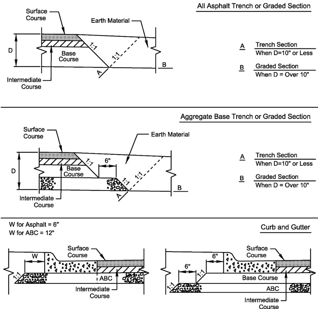
Figure 2-4 Pavement Edge Construction with Shoulder Drains
