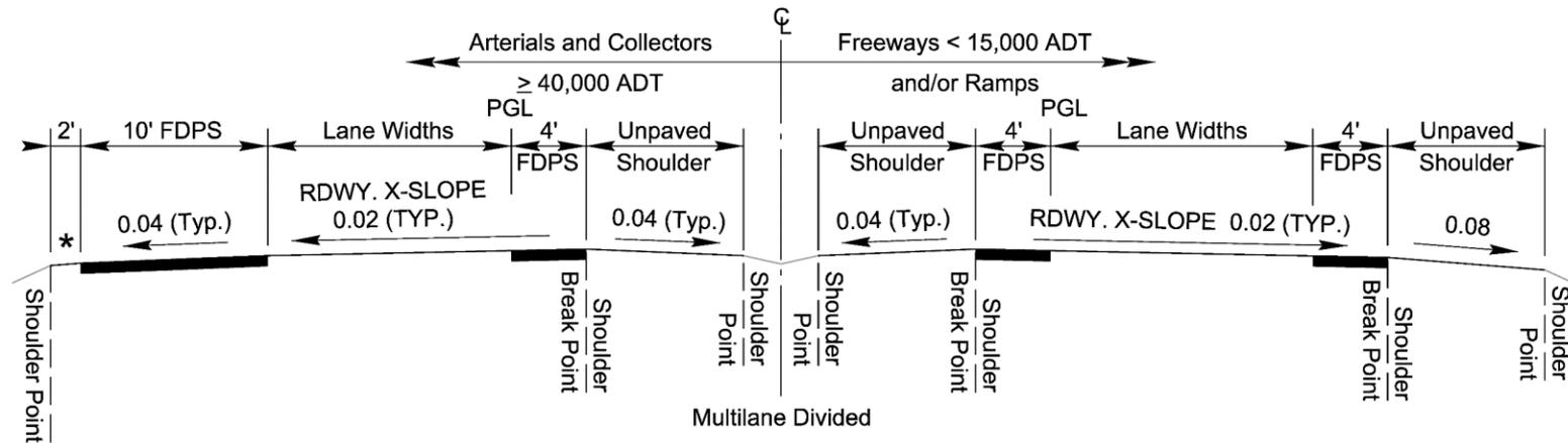
Figure 4-3 Typical Shoulder Cross Slopes (cont.)
