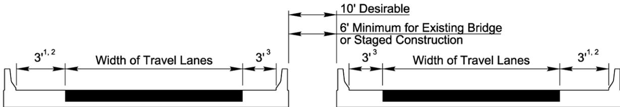
**Single Structure - Curb and Gutter Approach<sup>6,7</sup>**
