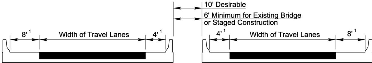
Single Structure - Curb and Gutter Approach<sup>3,4</sup>
