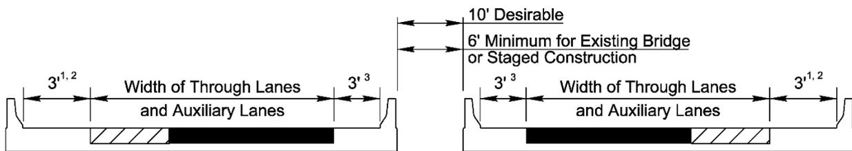
Single Structure - Curb and Gutter Approach<sup>6,7</sup>
