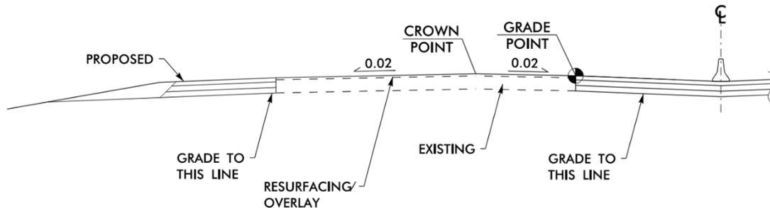
Draw typical sections for each different pavement design and for major variations in the component widths. Use partial typical sections or insets with notes for minor variations to minimize the number of typical sections required. Make a conscious effort to minimize the number of typical sections. The use of a single typical section to represent multiple alignments is encouraged. Use tables to denote the variations in dimension widths and pavement codes.
