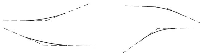
Note: Angular breaks to be appropriately rounded as shown (see text)
