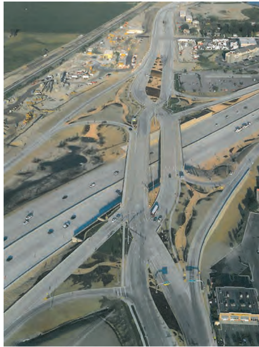
Exhibit 1-2. First constructed DDI in Utah at Pioneer Crossing and Interstate 15 (American Fork, Utah) (1).
