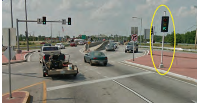
Exhibit 7-21. Supplemental signal on right for an inbound movement at a DDI (2).
