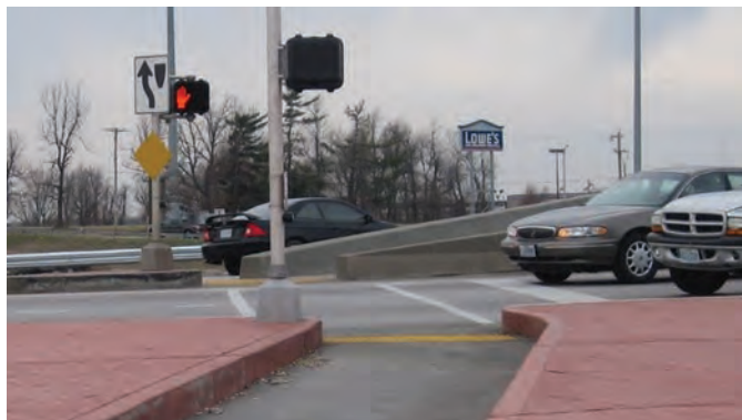
Exhibit 7-27. Pedestrian signal and push button on outside of crossover (pedestrian facility in median).
