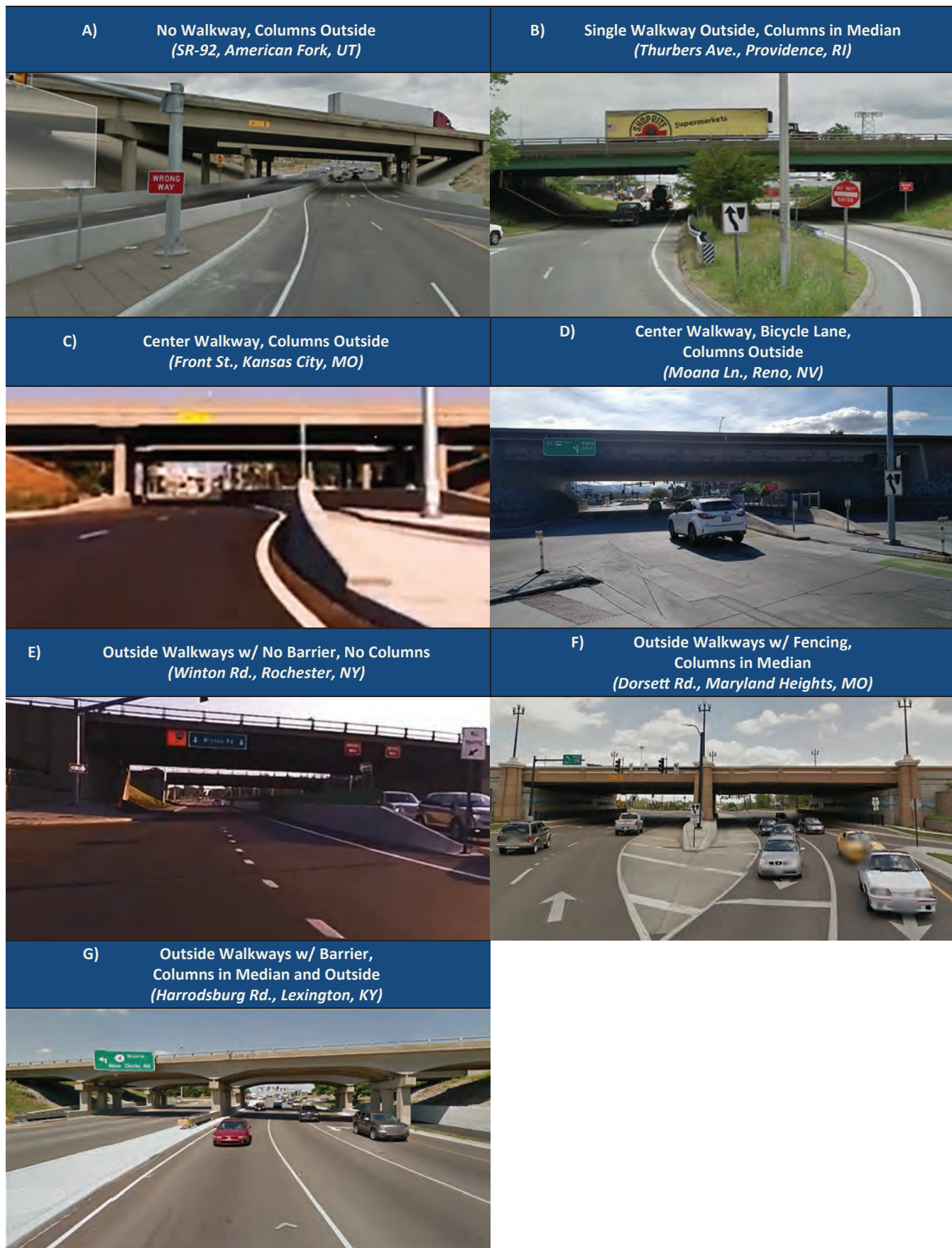
Exhibit 6-47. Examples of various underpass cross sections (3).
