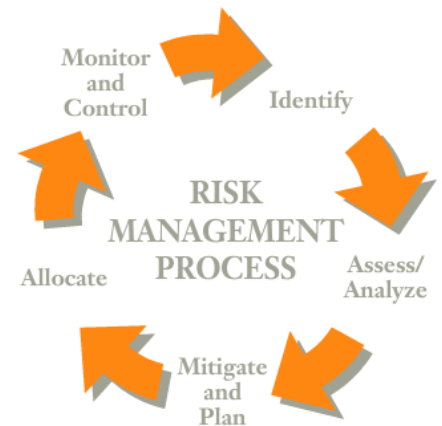
Figure 5, Cyclical Nature of Risk Management Process Risk Assessment and Allocation for Highway Construction Management
