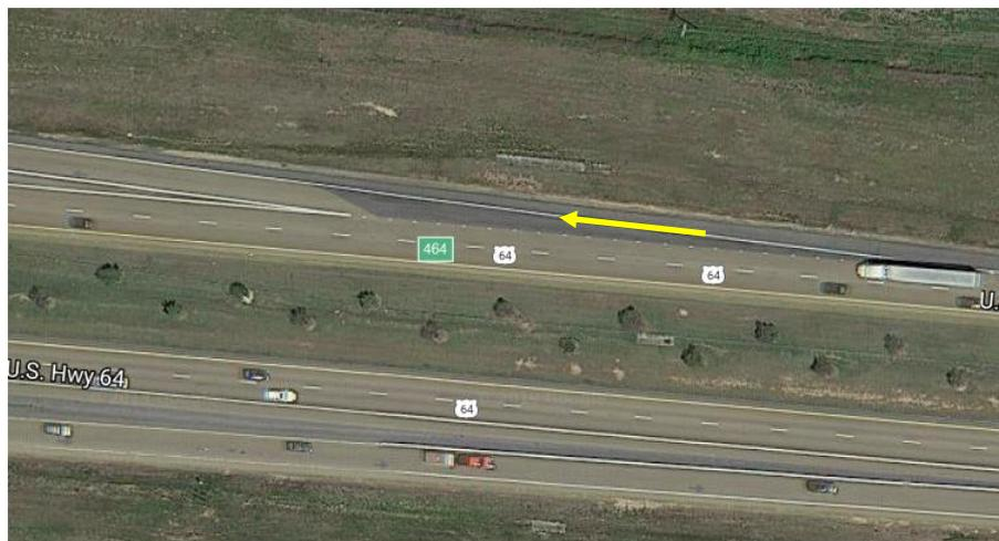
When coding a tapered exit on the freeway, after including a deceleration lane that starts where the taper is 8 feet wide, the ramp should diverge from the freeway where the edge of travel lines diverge, meaning that the tail of the lane connector arrows should start at this location (red arrow).
