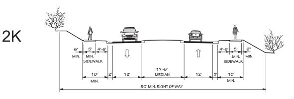
2 LANE DIVIDED (17'-6" RAISED MEDIAN) WITH CURB & GUTTER AND SIDEWALKS POSTED SPEED 25-45 MPH
