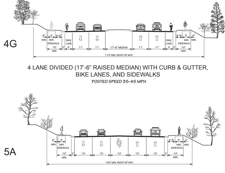
4 LANE WITH TWO WAY LEFT TURN LANE, CURB & GUTTER, AND SIDEWALKS POSTED SPEED 35-45 MPH
