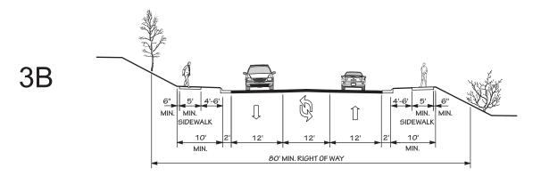
2 LANE WITH TWO WAY LEFT TURN LANE, CURB & GUTTER, AND SIDEWALKS POSTED SPEED 25-45 MPH
