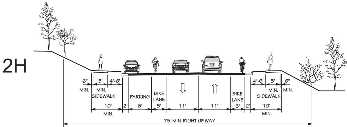
2 LANE UNDIVIDED WITH CURB & GUTTER, PARKING ONE SIDE, BIKE LANES, AND SIDEWALKS
