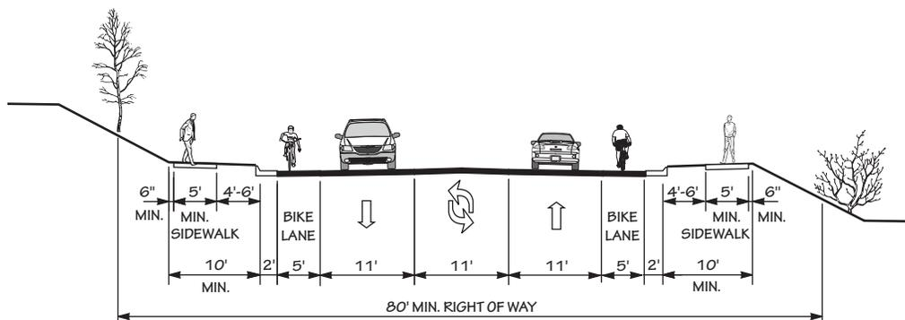
2 LANE WITH TWO WAY LEFT TURN LANE, CURB & GUTTER,
