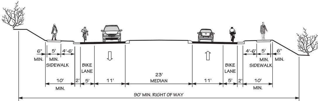
2 LANE DIVIDED (23' RAISED MEDIAN) WITH CURB & GUTTER, BIKE LANES, AND SIDEWALKS
