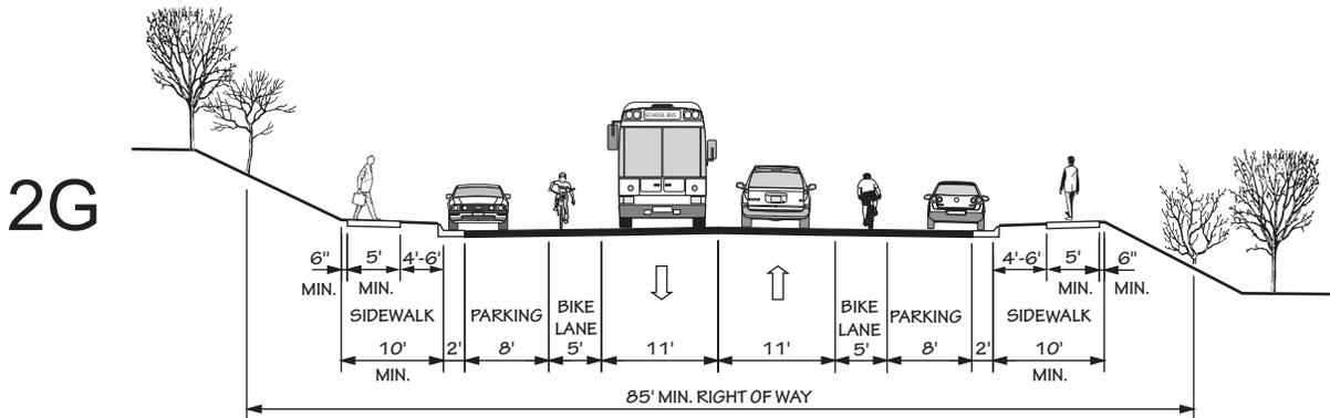
2 LANE UNDIVIDED WITH CURB & GUTTER, PARKING BOTH SIDES, BIKE LANES, AND SIDEWALKS
