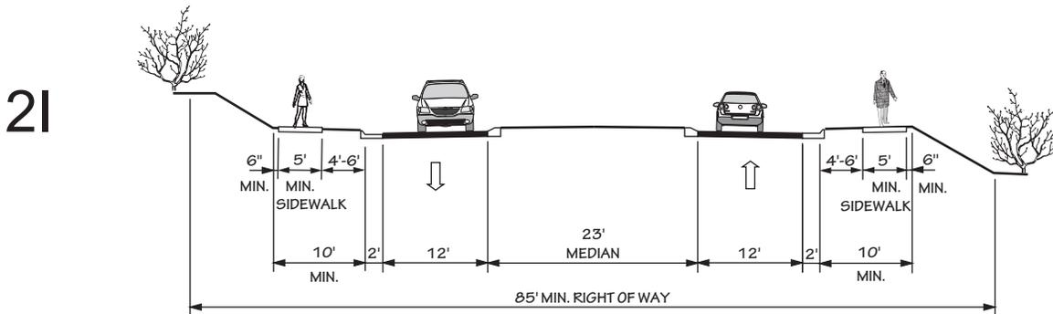
2 LANE DIVIDED (23' RAISED MEDIAN) WITH CURB & GUTTER AND SIDEWALKS
