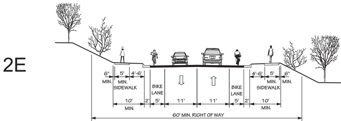
2 LANE UNDIVIDED WITH CURB & GUTTER, BIKE LANES, AND SIDEWALKS
