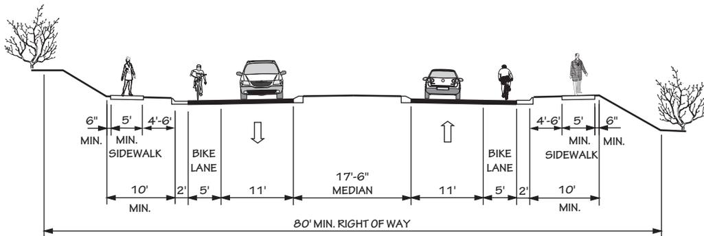
2 LANE DIVIDED (17'-6" RAISED MEDIAN) WITH CURB & GUTTER, BIKE LANES, AND SIDEWALKS
