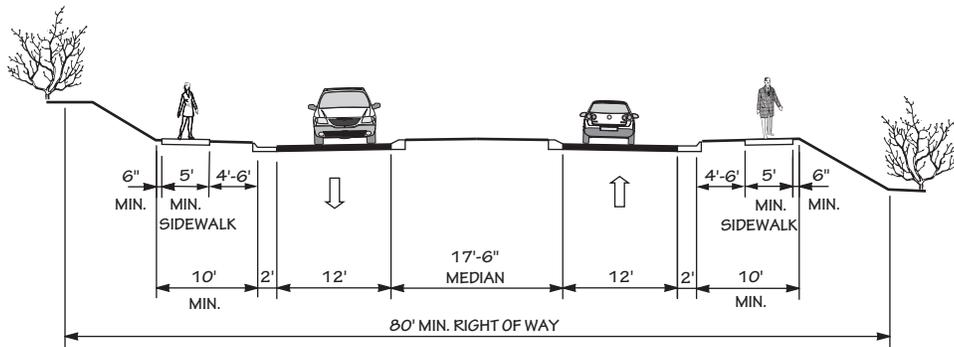
2 LANE DIVIDED (17'-6" RAISED MEDIAN) WITH CURB & GUTTER AND SIDEWALKS
