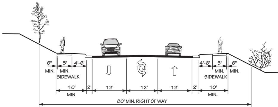
2 LANE WITH TWO WAY LEFT TURN LANE, CURB & GUTTER,
