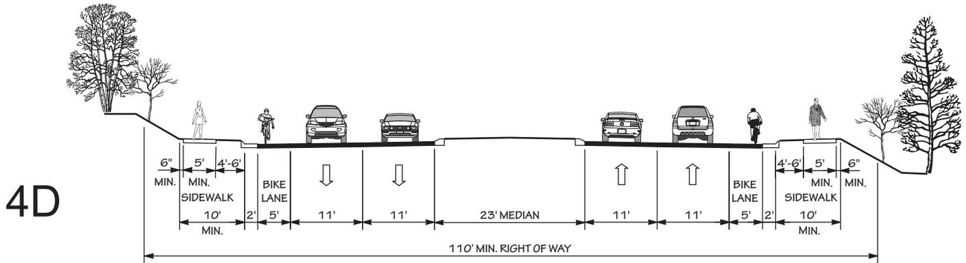
**4 LANE DIVIDED (23' RAISED MEDIAN) WITH CURB & GUTTER, BIKE LANES AND SIDEWALKS**
